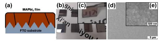
Fig. 1 The MAPbl<sub>3</sub> film deposited on the substrate: (a) schematic diagram, (b) and (c) photograph appearance, and (d) and (e) scanning electron microscope images under high and low resolutions.
