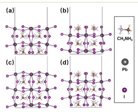
Fig. 3 The four possible surfaces of the MAPbl $_3$  crystal are stoichiometric atom ratio with MAI-termination (a) and with Pbl $_2$ -termination (b), and nonstoichiometric atom ratio with MAI-termination (c) and with Pbl $_2$ -termination (d).
