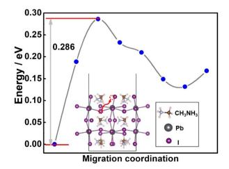
Fig. 5 The diffusion energy of  $I^-$  in the MAPbI<sub>3</sub> surface. The inset figure is the diffusion path of  $I^-$  when I vacancy defects exist.
