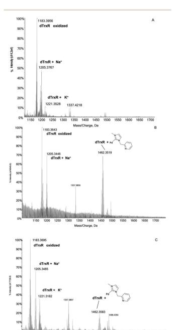
Fig. 3 (A) ESI mass spectra of dTrxR  $5\times10^{-7}$  M incubated at 37 °C for 2 h with (B) 3 and (C) 4 at 1 : 3:10 peptide-to-palladium-to-DTT ratio. 0.1% v/v of formic acid was added just before infusion.
