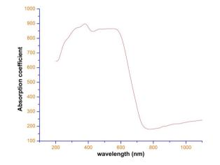
Fig. 9 Absorption coefficient vs. wavelength plot of DSFS crystal.
