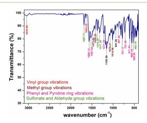
Fig. 6 FTIR spectrum of the grown DSFS crystal.
