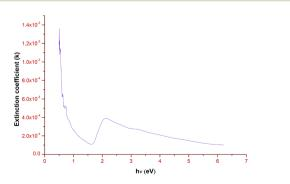
Fig. 10 Extinction coefficient vs. photon energy plot of DSFS crystal.
