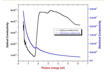
Fig. 11 Optical conductivity and electrical conductivity vs. photon energy plot.
