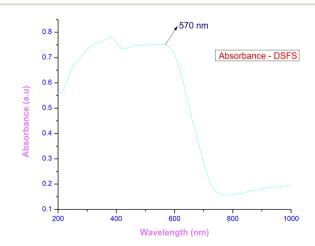
Fig. 7 Absorbance spectrum of the DSFS crystal.
