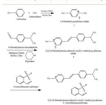
Fig. 1 Reaction scheme for the DSFS material.
