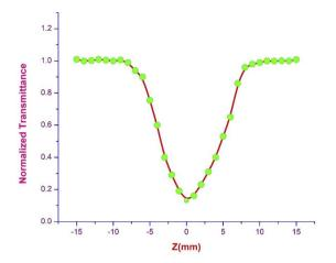
Fig. 17 Open aperture trace of DSFS crystal
