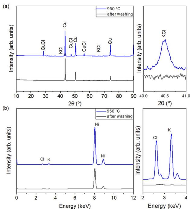
Fig. 6 (a) XRD and (b) XRF of the KCl-coated Cu NPs with the coating temperatures of 950 °C and after NH<sub>4</sub>OH washing.
