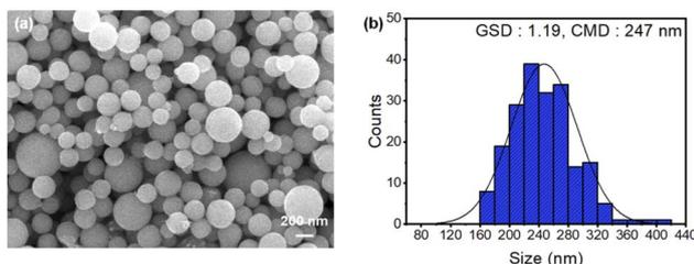
**Fig. 7** (a) FESEM image and (b) particle size distribution histogram of the KCl-coated Cu NPs after NH<sub>4</sub>OH washing.
