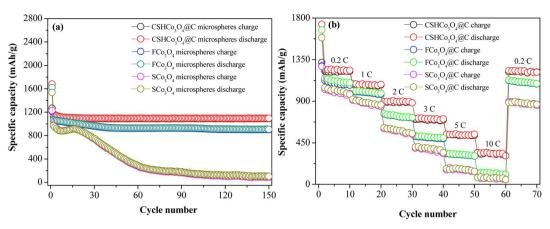
Fig. 5 (a) Cycling stability and (b) rate performance of the CSHCo<sub>3</sub>O<sub>4</sub>@C, SCo<sub>3</sub>O<sub>4</sub>, and FCo<sub>3</sub>O<sub>4</sub> microspheres
