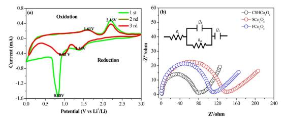
Fig. 6 (a) Cyclic voltammetry curves of the first 3 cycles of the  $CSHCo_3O_4@C$  microspheres and (b) electrochemical impedance spectroscopy results of the  $CSHCo_3O_4@C$ ,  $SCo_3O_4$ , and  $FCo_3O_4$  microspheres.
