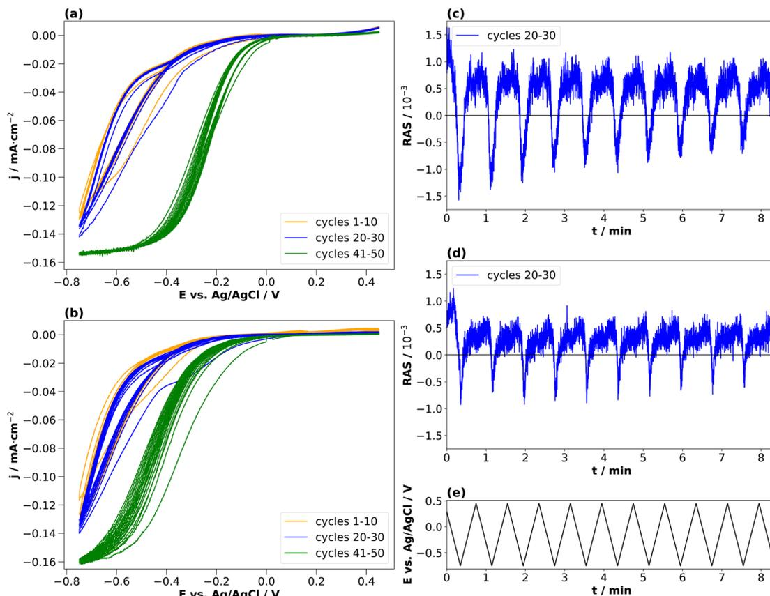
Fig. 5 Cyclic voltammograms of InP (a) HCl (0.5 M) and (b) H<sub>2</sub>SO<sub>4</sub> (0.25 M) with corresponding transients at 2.25 eV for cycles 20–30 (c and d) and the applied potentials (e). Potential plotted against Ag/AgCl. Scan from open-circuit potential towards  $-0.75$  V and then to  $+0.45$  V with a scan rate of  $0.05$  V s<sup>-1</sup>. The orange curve shows the cycles 1–10, the blue curve shows the cycles 20–30, and the green curve shows the cycles 41–50.
