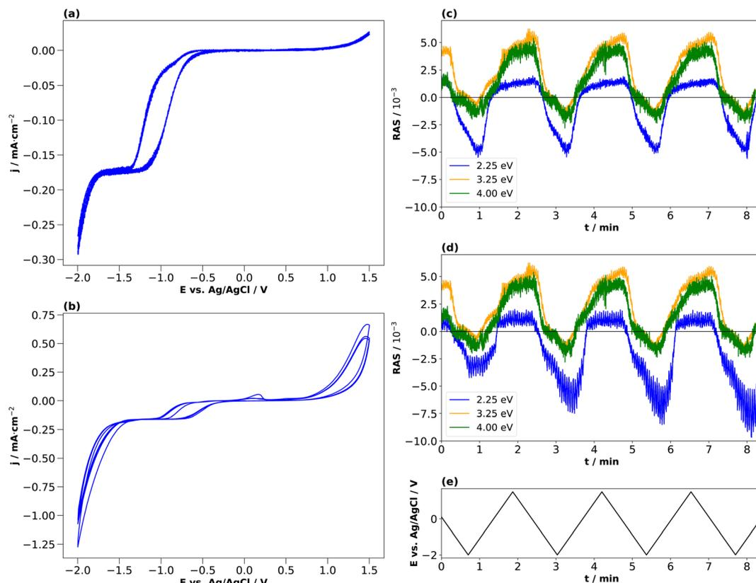
Fig. 4 Cyclic voltammograms of InP in 0.01 M (a) HCl with associated transients (c), and in 0.01 M (b) H<sub>2</sub>SO<sub>4</sub> with associated transients (d). (e) Potential plotted against Ag/AgCl. Scan from OCP towards -2 V and then to 1.5 V for 3 cycles, with a scan rate of 0.05 V s<sup>-1</sup>.
