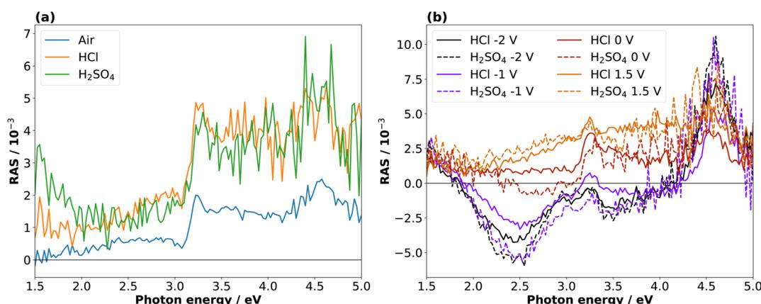
Fig. 2 (a) RA spectra of epi-ready InP(100) in air and immersed in 0.01 M HCl and H<sub>2</sub>SO<sub>4</sub> at open-circuit potential. (b) RA spectra at  $-2$  V,  $-1$  V,  $0$  V and  $1.5$  V of the InP(100) surface in 0.01 M HCl (solid line) and 0.01 M H<sub>2</sub>SO<sub>4</sub> (dashed line) solution.
