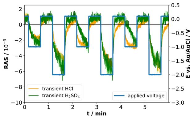
Fig. 6 Potential-step and transient measurements at 2.25 eV in 0.01 M HCl and in 0.01 M H<sub>2</sub>SO<sub>4</sub>.
