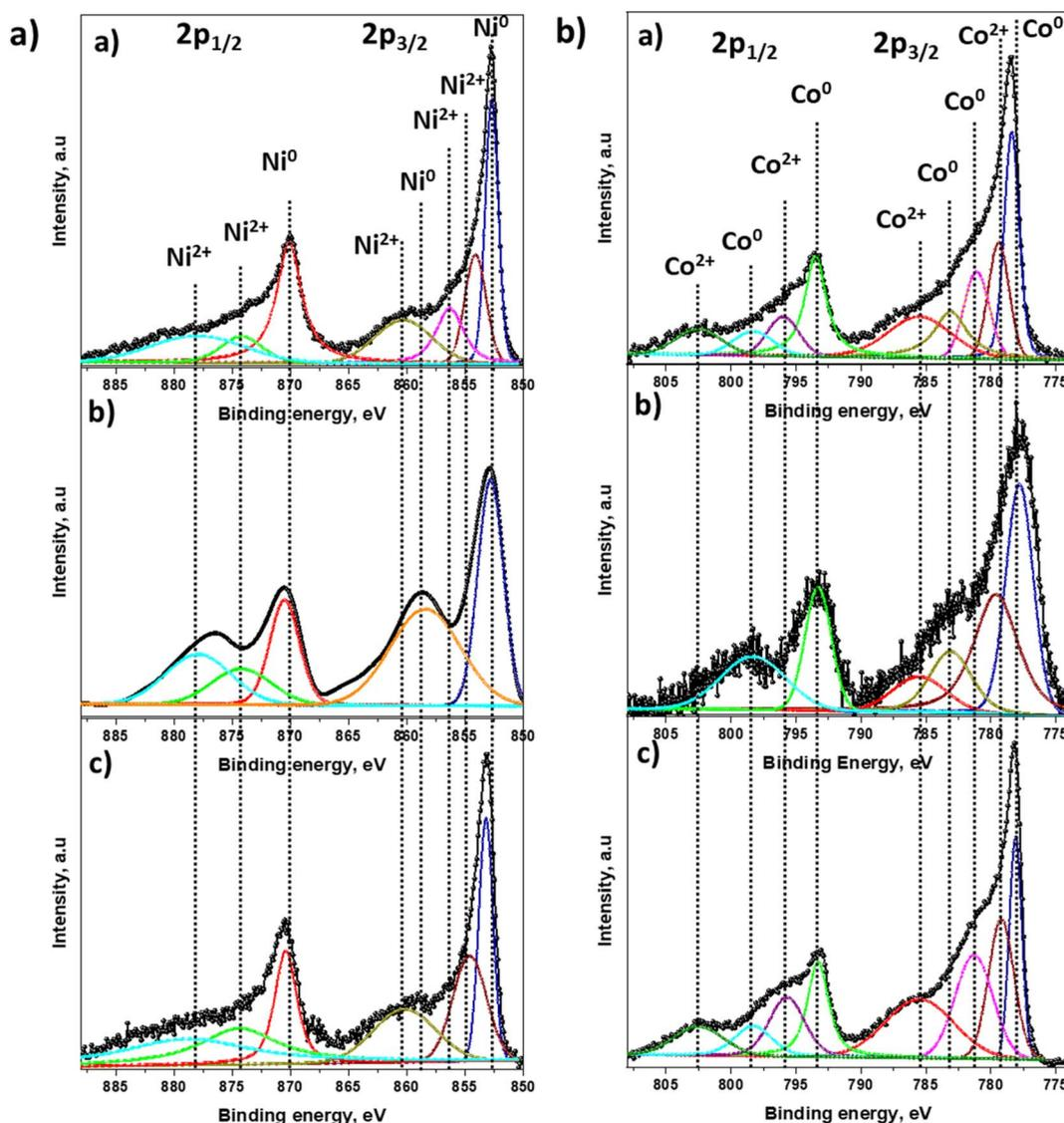
Fig. 3 HR-XPS spectra of (a) Ni 2p; (b) Co 2p. Insight (a)–(c) represents Ni<sub>6</sub>Co<sub>4</sub>-AC, Ni<sub>5</sub>Co<sub>5</sub>-AC and Ni<sub>4</sub>Co<sub>6</sub>-AC.
