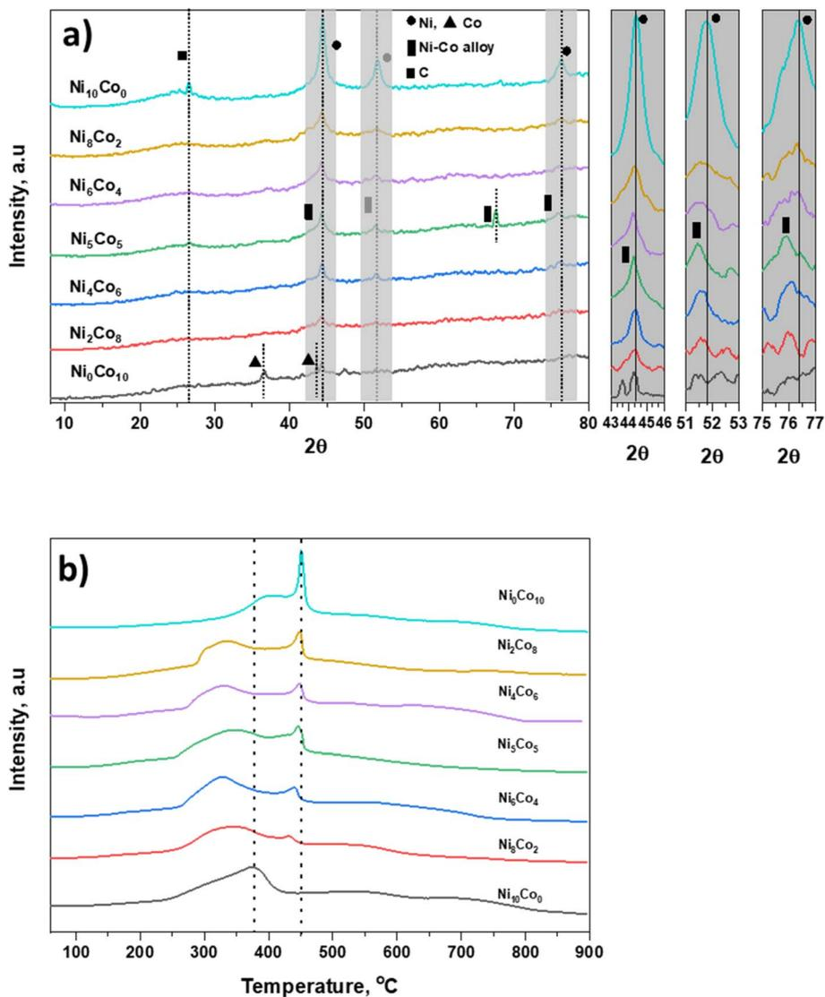
Fig. 1 (a) P-XRD pattern; (b) H<sub>2</sub>-TPR profile of activated carbon supported NiCo-AC catalysts.
