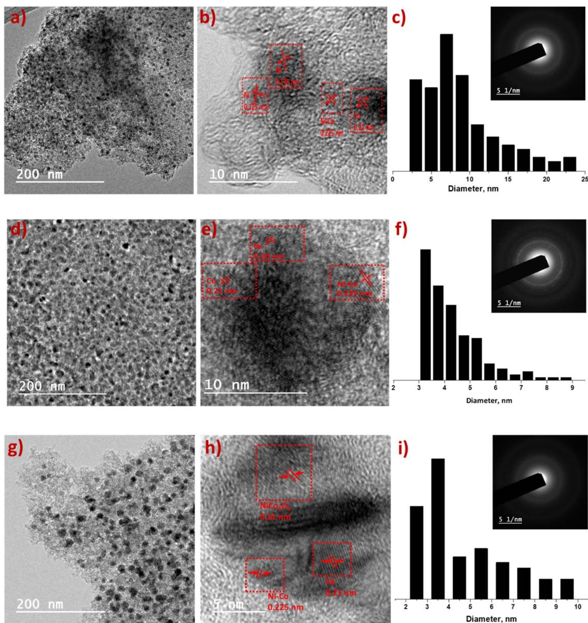
Fig. 2 HR-TEM images of Ni<sub>6</sub>Co<sub>4</sub>-AC (a–c), Ni<sub>5</sub>Co<sub>5</sub>-AC (d–f) and Ni<sub>4</sub>Co<sub>6</sub>-AC (g–i). (b, e and h) interplanar *d*-spacing in high magnified TEM; (c, f and i) particle size range of metals and SAED pattern.
