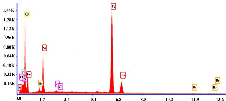
Fig. 5 The EDS analysis of SMNPs@DABCO@eosin.
