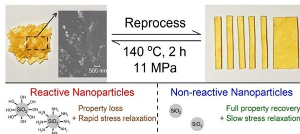
Fig. 5 Reprocessable polyhydroxyurethane network nanocomposites using silica nanoparticles with different surface functionalities as reinforcing fillers.<sup>68</sup>
