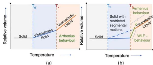
Fig. 3 Temperature dependent phase transitions of vitrimers. (a)  $T_g$  below  $T_v$  and (b)  $T_g$  above  $T_v$ .<sup>34</sup>
