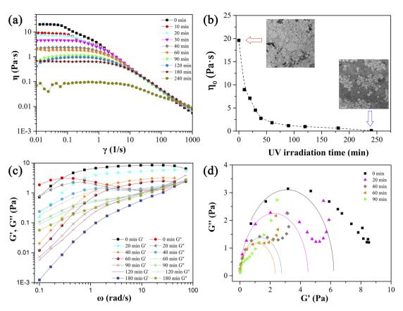
Fig. 10 The steady viscosity curves (a), zero-shear viscosities (b), dynamic viscoelastic modulus (c) and Cole-Cole plots (d) of 28 mM 12-3(OH)- $12\cdot2Br^{-}/12$  mM trans-OHCA mixed solution before and after UV irradiation for different time at 25 °C.
