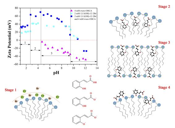
Fig. 9 The supposed self-assembly behavior of  $12-3(OH)-12\cdot 2Br^-/trans$ -OHCA in different pH according to the zeta potentials. Stage 1: pH < 2.7; stage 2: pH 2.7–4.5; stage 3: pH 4.5–9.6; stage 4: pH > 9.6.
