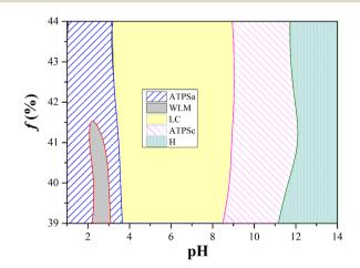
Fig. 7 The pH regions of different aggregates formed by 12-3(OH)-12·2Br<sup>-</sup>/trans-OHCA when changed the molar percentage of trans-OHCA of 39% to 44% and kept the solution concentration as 50 mM. ATPSa: the aqueous two phase system in acid conditions; WLM: wormlike micelles; LC: liquid crystals; ATPSc: the aqueous two phase system in alkaline condition; H: weak hydrogel.
