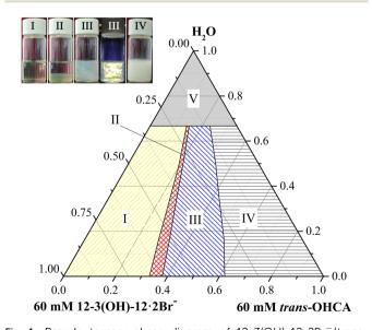
Fig. 1 Pseudo ternary phase diagram of  $12-3(OH)-12\cdot2Br^-/trans-OHCA/H_2O$  mixed system at 40 °C. (I) micellar phase; (II) aqueous two phase system, ATPS; (III) lamellar liquid crystal phase; (IV) precipitate; (V) unmeasured areas.
