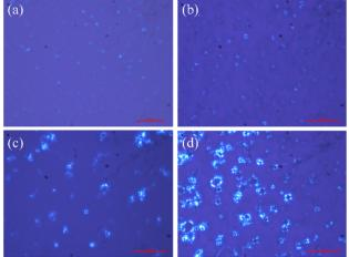
Fig. 5 The polarized microscopy images of the liquid crystals formed by 30 mM 12-3(OH)-12·2Br<sup>-</sup>/20 mM trans-OHCA in different pH at 40 °C. (a): pH 4.32; (b): pH 6.47; (c): pH 7.94; (d): pH 8.75.
