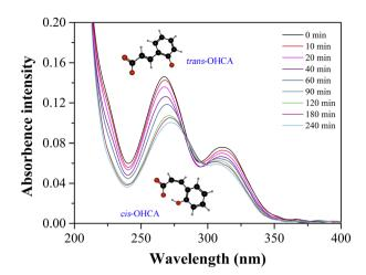
Fig. 11 The UV-vis absorption spectra of  $0.14 \text{ mM } 12-3(OH)-12\cdot 2Br^-/0.06 \text{ mM } trans-OHCA$  after UV irradiation for different time.
