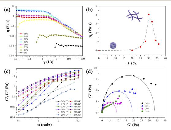
Fig. 2 The influences of *trans*-OHCA molar percentage on the steady viscosity curves (a), zero-shear viscosity (b), dynamic viscoelastic modulus (c) and corresponding Cole–Cole plots (d) of micellar solutions formed in 12-3(OH)- $12\cdot2$ Br $^-$ /trans-OHCA/H $_2$ O system at 40 °C. The total concentration of these solutions was maintained at 40 mM and the legends referred to the molar percentages of *trans*-OHCA in the solution.
