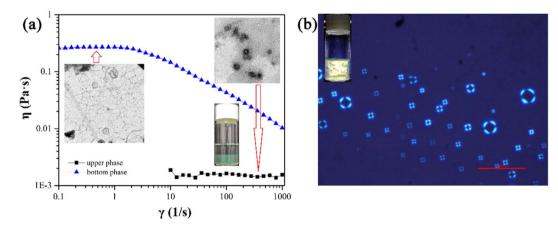
Fig. 3 The viscosity curves and TEM images of the ATPS (a) as well as the polarized microscopy image of liquid crystals (b) formed in 12-3(OH)-12.2Br<sup>-</sup>/trans-OHCA/H<sub>2</sub>O mixed system at 40 °C.
