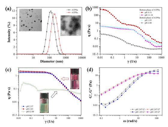
Fig. 6 The size distributions and TEM images of aggregates formed in the upper phase of ATPSa and ATPSc (a), the viscosity curves of the bottom phases of the ATPSa and ATPSc (b), the viscosity curves of wormlike micellar solution and the weak hydrogel (c), and the elastic modulus and viscous modulus of wormlike micelles (d). All these phases were formed by 30 mM 12-3(OH)- $12\cdot2$ Br $^-$ /20 mM trans-OHCA in different pH at 40 ° C
