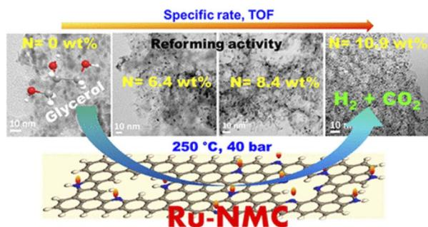
Fig. 7 Schematic of the experiment for enhanced H<sub>2</sub> production through the aqueous-phase reforming of glycerol.<sup>110</sup>
