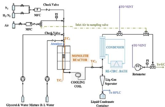
Fig. 6 Schematic of experimental set-up.<sup>96</sup>
