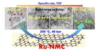
Fig. 7 Schematic of the experiment for enhanced  $\rm H_2$  production through the aqueous-phase reforming of glycerol.  $^{110}$
