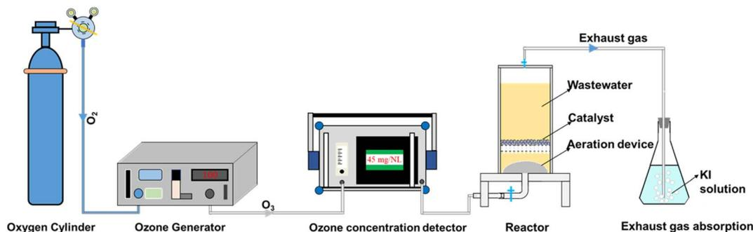
Fig. 1 Experimental apparatus and the catalytic ozonation system.
