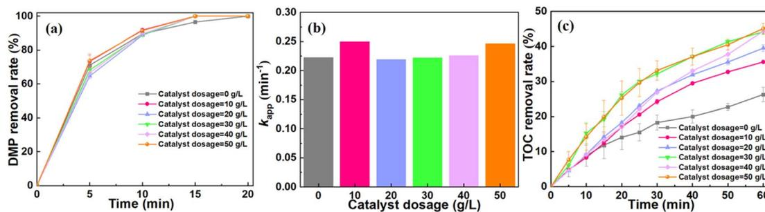
Fig. 3 Effect of catalyst dosage on DMP removal efficiency. (a) The DMP removal rate under the conditions of different catalyst dosages; (b) the  $k_{app}$  of DMP degradation at different catalyst dosages; (c) the removal rate of TOC at different catalyst dosages. Experimental conditions: ozone dosage = 22.5 mg min<sup>-1</sup>, pH = 6, [DMP]<sub>0</sub> = 70 mg L<sup>-1</sup>.
