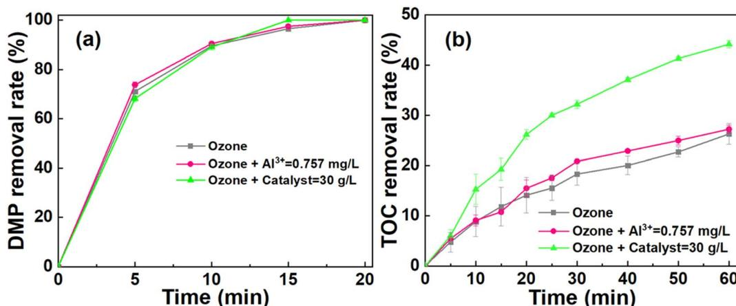
Fig. 7 The effect of dissolved ions on DMP degradation. (a) The effect on DMP removal rate. (b) The effect on TOC removal rate. Experimental conditions: catalyst dosage = 30 g L<sup>-1</sup>, ozone dosage = 22.5 mg min<sup>-1</sup>, pH = 6, [DMP]<sub>0</sub> = 70 mg L<sup>-1</sup>, [Al<sup>3+</sup>]<sub>0</sub> = 0.757 mg L<sup>-1</sup>.
