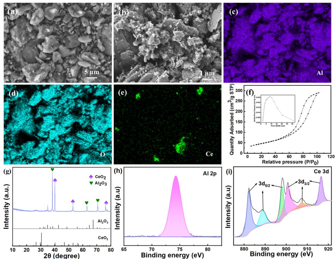
Fig. 2 SEM images, elemental mappings, BET test, XRD patterns and XPS tests of the  $\text{CeO}_2/\text{Al}_2\text{O}_3$  catalyst. SEM image at  $1000\times$  magnification (a) and  $8000\times$  magnification (b); EDS mapping of Al (c), O (d) and Ce (e); BET test (f); XRD patterns (g); XPS tests (h) and (i).
