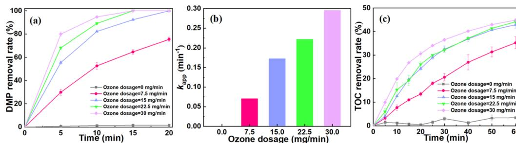
Fig. 4 Effect of ozone dosage on DMP removal efficiency. (a) The DMP removal rate under the conditions of different ozone dosages; (b) the  $k_{app}$  of DMP degradation at different ozone dosages; (c) the removal rate of TOC in the system at different ozone dosages. Experimental conditions: catalyst dosage = 30 g L<sup>-1</sup>, pH = 6, [DMP]<sub>0</sub> = 70 mg L<sup>-1</sup>.
