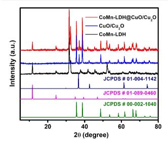
Fig. 1 Comparison of powder XRD patterns of CoMn-LDH, CuO/Cu $_2$ O and CoMn-LDH $_0$ CuO/Cu $_2$ O.
