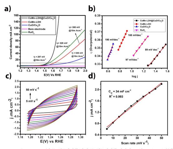
Fig. 4 (a) Linear sweep voltammograms of CoMn-LDH, CuO/Cu<sub>2</sub>O, CoMn-LDH@CuO/Cu<sub>2</sub>O, RuO<sub>2</sub> and B are electrode (b) Tafel slopes of CoMn-LDH, CuO/Cu<sub>2</sub>O, CoMn-LDH@CuO/Cu<sub>2</sub>O and RuO<sub>2</sub> (c) non-faradaic region cyclic voltammograms at various scan rates (d) anodic current density plot vs. scan rate of CoMn-LDH@CuO/Cu<sub>2</sub>O fabricated electrode in 1 M KOH solution as an electrolyte.
