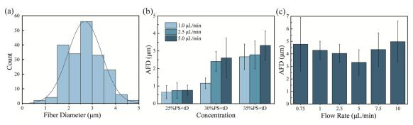
Fig. 4 (a) Histogram of fiber diameter distribution of electrospun fibers prepared with PS solution concentration of 35 wt% at a flow rate of 1.0  $\mu$ L min<sup>-1</sup>. Average fiber diameter of the SMP electrospun fibers with different PS solution concentrations at various flow rates, (b) tD/PS (25, 30, and 35 wt%), and (c) tD/PS (40 wt%).
