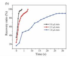
Fig. 6 (a) The digital images of the shape memory effect process of the bended tD/PS (35 wt%) electrospun web using 5  $\mu$ L min<sup>-1</sup> flow rate at 70 °C; (b) the shape recovery ratios as a function of the heating time for electrospun fibers with PS solution concentration of 35 wt% at various flow rates (1.0; 2.5 and 5.0  $\mu$ L min<sup>-1</sup>).
