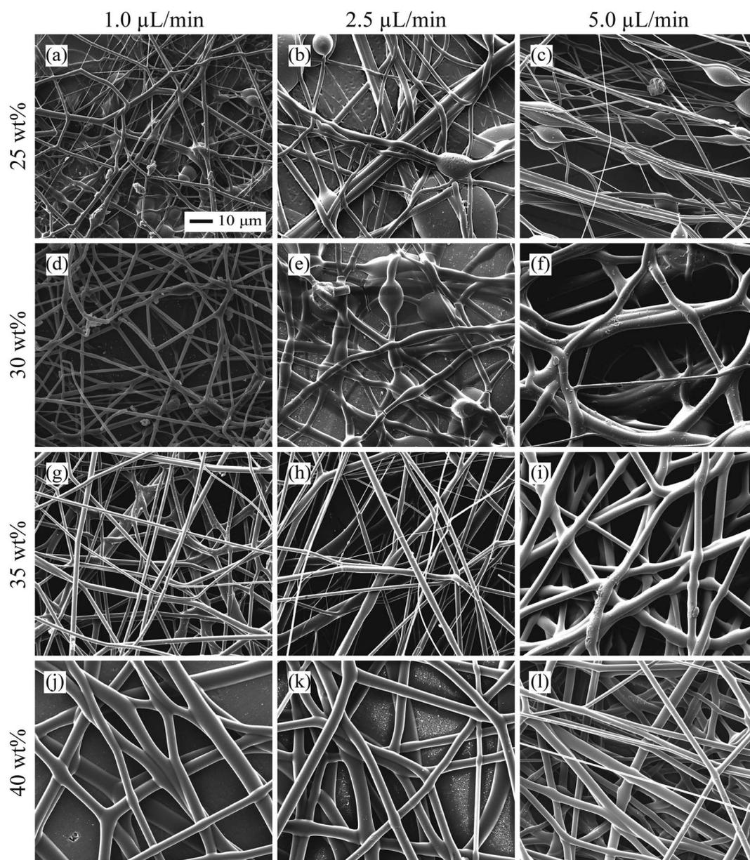
Fig. 3 SEM pictures ( $\times 1K$  magnification) of SMP electrospun fibers with different PS solution concentrations of 25 wt% (a–c), 30 wt% (d–f), 35 wt% (g–i) and 40 wt% (j–l) at various flow rates of 1.0  $\mu\text{L min}^{-1}$  (a, d, g, j), 2.5  $\mu\text{L min}^{-1}$  (b, e, h, k) and 5.0  $\mu\text{L min}^{-1}$  (c, f, i, l).
