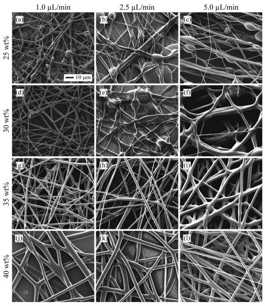
Fig. 3 SEM pictures ( $\times$ 1K magnification) of SMP electrospun fibers with different PS solution concentrations of 25 wt% (a–c), 30 wt% (d–f), 35 wt% (g–i) and 40 wt% (j–l) at various flow rates of 1.0  $\mu$ L min<sup>-1</sup> (a, d, g, j), 2.5  $\mu$ L min<sup>-1</sup> (b, e, h, k) and 5.0  $\mu$ L min<sup>-1</sup> (c, f, i, l).
