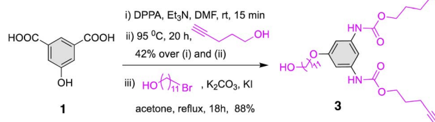
Scheme 1 Synthesis of dendron 3 using one-pot multicomponent Curtius reaction followed by the spacer group attachment.
