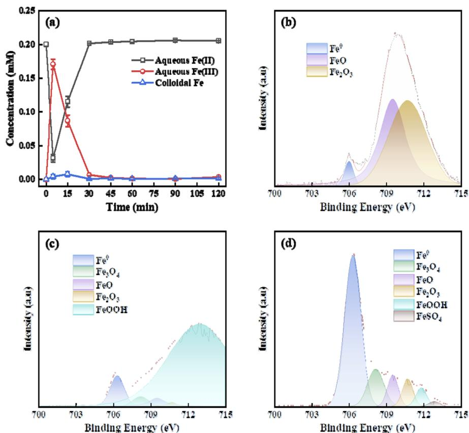
Fig. 4 (a) Changes of Fe species in homogeneous solution of FEEF system, XPS spectrums of Fe species on (b) pristine steel mesh, (c) FESSM cathode after electrochemical experiment, (d) FESSM cathode after electrochemical experiment and cleaning the Fe sludge adsorbed on cathode surface. Experimental conditions:  $[PTSA]_0 = 100 \text{ mg L}^{-1}$ , applied voltage = 2.5 V, pH = 3.0, 0.2 mM  $\text{Fe}^{2+}$  and 1.0 mM  $\text{H}_2\text{O}_2$  dosage.
