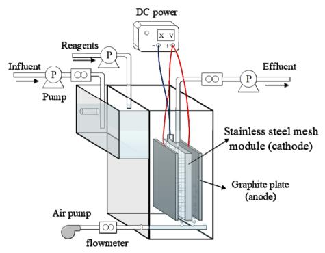
Fig. 1 Schematic of filtration-enhanced electro-Fenton (FEEF) experimental setup.
