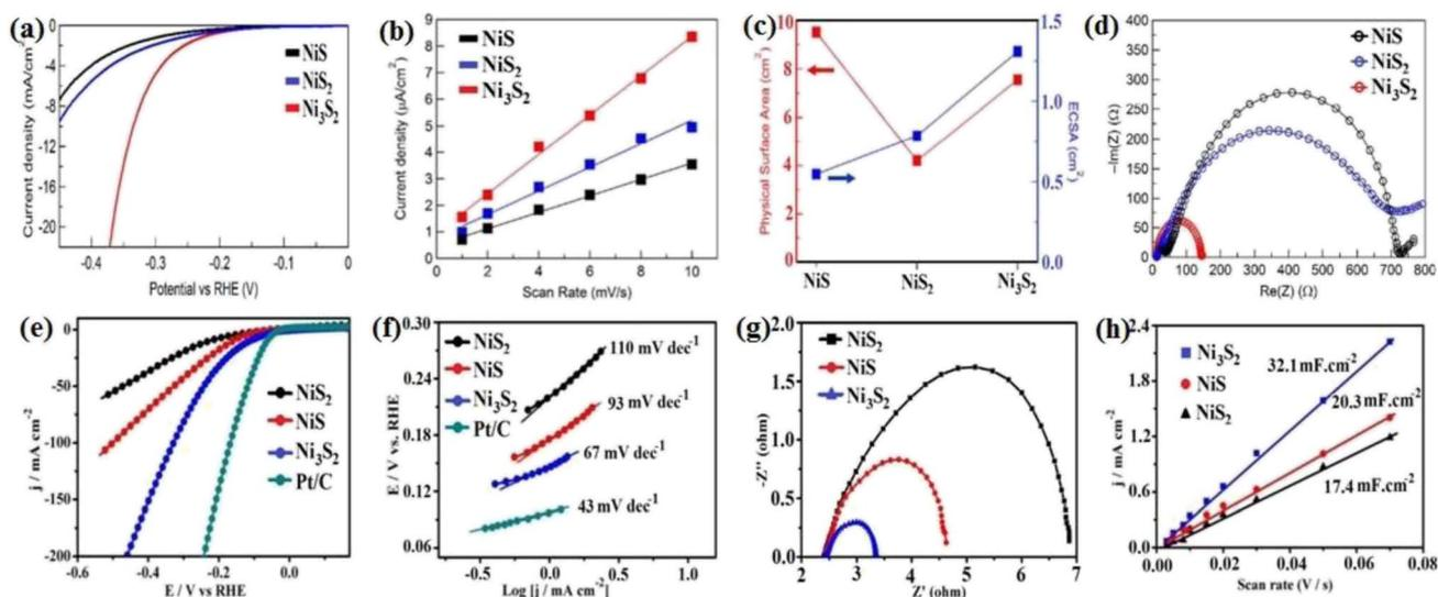
Fig. 8 Ni<sub>3</sub>S<sub>2</sub>, NiS and NiS<sub>2</sub> electrocatalysts: (a) LSV curves in 1.0 M KOH, (b) electrochemical double-layer capacitance, (c) comparison of SSA (red) and ECSA (blue),<sup>49</sup> (d) EIS, (e) LSV curves in 1.0 M KOH, (f) corresponding Tafel plots, (g) EIS plots and (h) electrochemical double-layer capacitance.<sup>80</sup>
