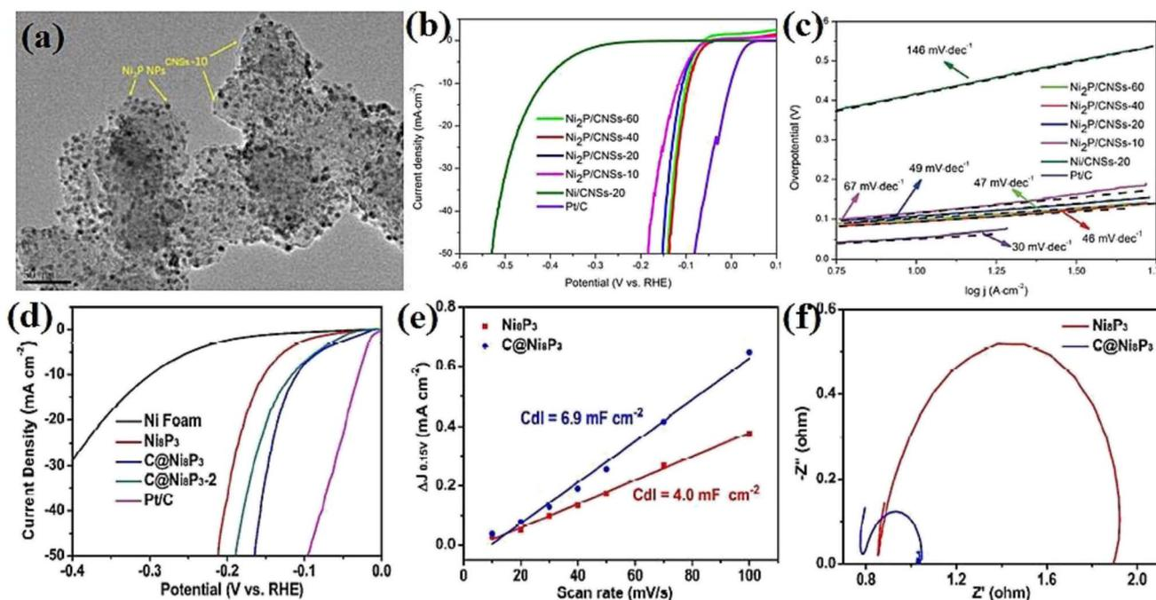
Fig. 14 Ni<sub>2</sub>P supported on carbon nanospheres: (a) TEM image, (b) LSV curves in 0.5 M H<sub>2</sub>SO<sub>4</sub> and (c) corresponding Tafel plots (reproduced from ref. 78 with permission from Elsevier, Copyright 2015). Carbon-coated Ni<sub>8</sub>P<sub>3</sub>: (d) LSV curves in 0.5 M H<sub>2</sub>SO<sub>4</sub>, (e) electrochemical double-layer capacitance and (f) EIS plots (reproduced from ref. 108 with permission from the America Chemistry Society, Copyright 2016).
