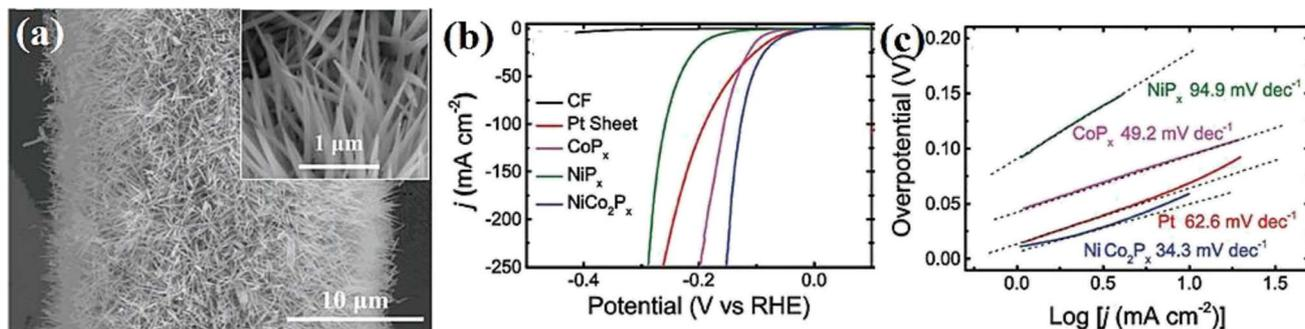
Fig. 12 NiCo<sub>2</sub>P<sub>x</sub> nanowire arrays: (a) SEM image, (b) LSV curves in 1.0 M KOH and (c) corresponding Tafel plots (reproduced from ref. 111 with permission from Wiley, Copyright 2017).
