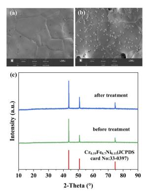
Fig. 2 Surface morphology of the FSS: (a) before treatment; (b) after treatment; (c) XRD of the FSS.
