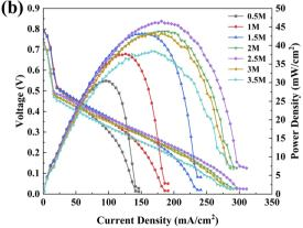
Fig. 4 Polarization curves of  $\mu DMFC$  with different structures at different methanol solution concentrations: (a) CCP-MEA; (b) FSS-MEA.
