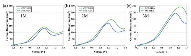
Fig. 5 Crossover current densities of  $\mu$ DMFCs at different methanol concentrations: (a) 1 mol L; (b) 2 mol L; (c) 3 mol L<sup>-1</sup>.
