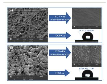
Fig. 3 Surface morphology and contact angle: (a) conventional carbon paper; (b) flotted stainless steal.
