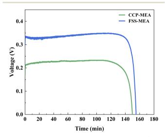
Fig. 9 Long-time discharge of  $\mu DMFCs$  at 343 K and 2 mol L<sup>-1</sup> under a discharge current density of 100 mA cm<sup>-2</sup>.
