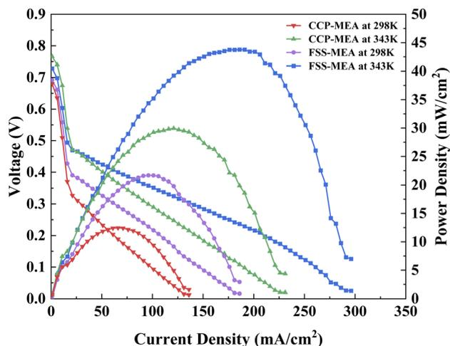
Fig. 6 Power density curves of  $\mu$ DMFC at different temperatures and 2 mol L<sup>-1</sup> methanol concentration.Table 4 Maximum power density of the two types of  $\mu$ DMFC at different temperatures
