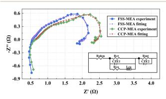
Fig. 8 EIS of  $\mu$ DMFCs at 343 K, 2 mol L<sup>-1</sup> and 80 mA cm<sup>-2</sup>.
