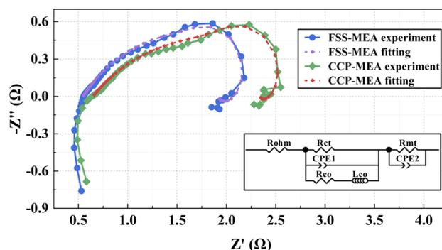
Fig. 8 EIS of  $\mu$ DMFCs at 343 K, 2 mol L<sup>-1</sup> and 80 mA cm<sup>-2</sup>.
