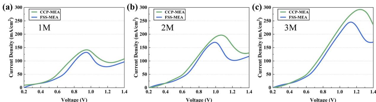
Fig. 5 Crossover current densities of  $\mu$ DMFCs at different methanol concentrations: (a) 1 mol L<sup>-1</sup>; (b) 2 mol L<sup>-1</sup>; (c) 3 mol L<sup>-1</sup>.
