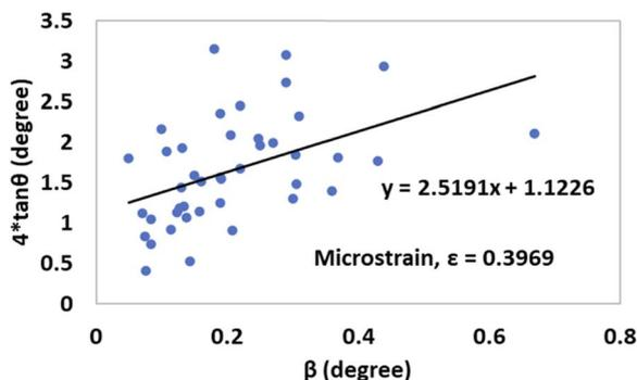
Fig. 12 Microstrain of gypsum using the straight-line model.
