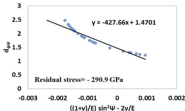
Fig. 15 Residual stress of bassanite employing the XRD- $\sin^2 \Psi$  technique.
