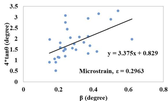
Fig. 13 Microstrain of bassanite using the straight-line model.
