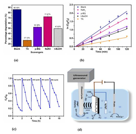
Fig. 5 (a) Scavenger study plot for the SEC oxidation of SMX on FTO/BaZr<sub>(0.1)</sub>Ti<sub>(0.9)</sub>O<sub>3</sub> electrode in the presence and absence of trapping agents, (b) reusability plot for the SEC oxidation of SMX on FTO/BaZr<sub>(0.1)</sub>Ti<sub>(0.9)</sub>O<sub>3</sub> electrode, (c) diagrammatic representation of the SEC oxidation system (d) proposed reaction scheme using FTO/BaZr<sub>(0.1)</sub>Ti<sub>(0.9)</sub>O<sub>3</sub> electrode.
