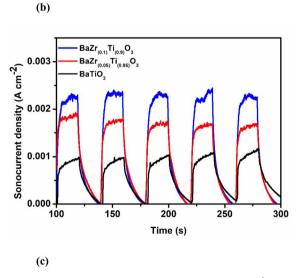
Fig. 2 (a) Cyclic voltammogram at scan rate of  $100 \text{ mV s}^{-1}$ , (b) Nyquist plot at  $10^5 \text{ Hz}$  to  $10^{-2} \text{ Hz}$  and bias potential of 0.21 V for all the prepared electrodes, (c) transient sonoelectrochemical current density response at 2.0 V bias potential.
