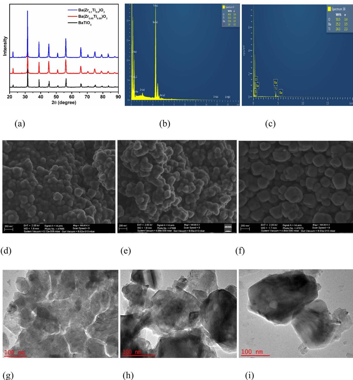
Fig. 1 (a) X-ray diffractogram of the piezoelectric materials, (b) EDS spectrum of  $\text{BaZr}_{(0.1)}\text{Ti}_{(0.9)}\text{O}_3$ , FESEM images of (c)  $\text{BaTiO}_3$  (d)  $\text{BaZr}_{(0.05)}\text{Ti}_{(0.95)}\text{O}_3$ , (e)  $\text{BaZr}_{(0.1)}\text{Ti}_{(0.9)}\text{O}_3$ , HRTEM images of (f)  $\text{BaTiO}_3$ , (g)  $\text{BaZr}_{(0.05)}\text{Ti}_{(0.95)}\text{O}_3$ , (h)  $\text{BaZr}_{(0.1)}\text{Ti}_{(0.9)}\text{O}_3$ , (i)  $\text{BaZr}_x\text{Ti}_{(1-x)}\text{O}_3$ .
