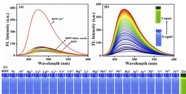
Fig. 2 (a) Fluorescence spectra of **BIPP** (2.0 M) after the addition of 21 metal ions (5 equiv.) in an ACN/ $\text{H}_2\text{O}$  (8 : 2, v/v) solution. (b) Fluorescent spectra of **BIPP** (2.0 M) in ACN/ $\text{H}_2\text{O}$  (8 : 2, v/v) solution with different  $\text{Zn}^{2+}$  ions concentrations (0–3 equivalent). (c) Fluorescence bottle images of **BIPP** in solution with various metal ions ( $1 \times 10^{-3}$  M).
