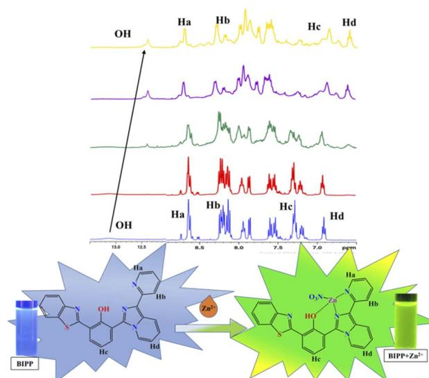
Fig. 4 <sup>1</sup>H NMR spectra of BIPP (400 MHz,  $\text{DMSO}-d_6$ , TMS) and the complex **BIPP**- $\text{Zn}^{2+}$  following the addition of  $\text{Zn}^{2+}$  ions.
