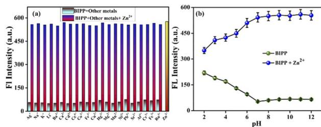
Fig. 3 (a) Competitive assays for the fluorescence responses of BIPP (1  $\mu\text{M}$ ) in the presence of  $\text{Zn}^{2+}$  ions (1  $\mu\text{M}$ ) and other competing metal ions (5  $\mu\text{M}$ ) in ACN/ $\text{H}_2\text{O}$  (8 : 2, v/v) solution. (b) In the absence and presence of  $\text{Zn}^{2+}$ , the influence of pH on the fluorescence intensity of BIPP in ACN/HEPES buffer (8 : 2) (pH 2.0–12.0) solutions.
