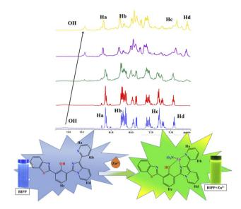
Fig. 4  $^{1}$ H NMR spectra of BIPP (400 MHz, DMSO-d<sub>6</sub>, TMS) and the complex BIPP-Zn<sup>2+</sup> following the addition of Zn<sup>2+</sup> ions.
