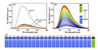
Fig. 2 (a) Fluorescence spectra of BIPP (2.0 M) after the addition of 21 metal ions (5 equiv.) in an ACN/H<sub>2</sub>O (8 : 2, v/v) solution. (b) Fluorescent spectra of BIPP (2.0 M) in ACN/H<sub>2</sub>O (8 : 2, v/v) solution with different  $Zn^{2+}$  ions concentrations (0–3 equivalent). (c) Fluorescence bottle images of BIPP in solution with various metal ions (1  $\times$  10<sup>-3</sup> M).
