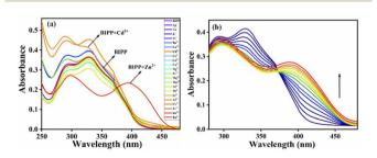
Fig. 1 (a) UV-Vis absorption spectra of sensor BIPP (1  $\times$  10<sup>-6</sup> M) towards 5 equiv. of various anions in ACN/H<sub>2</sub>O (8 : 2, v/v) solution; (b) absorption spectra of sensor BIPP (1  $\times$  10<sup>-6</sup> M) in ACN/H<sub>2</sub>O (8 : 2, v/v) solution upon the addition of various concentrations of Zn<sup>2+</sup> ions (0–2 equivalents).
