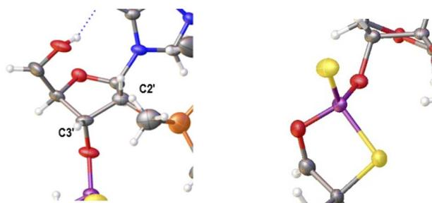
Fig. 2 Parts of the X-ray ORTEP diagram show: left image—a DNA-like C2'-*endo* conformation of detritylated *fast*-eluting **3a**; right image – spatial orientation of substituents on the phosphorus atom. Colors as in Fig. 1.
