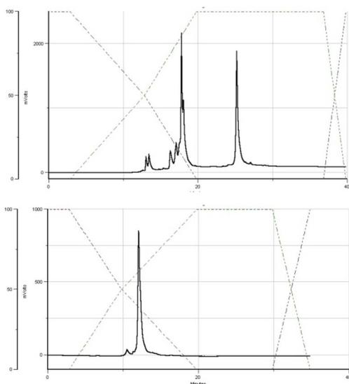
Fig. 4 HPLC profiles recorded for <sup>M</sup>GS during DMT-ON (the upper panel) and DMT-OFF (the lower panel) purification steps.
