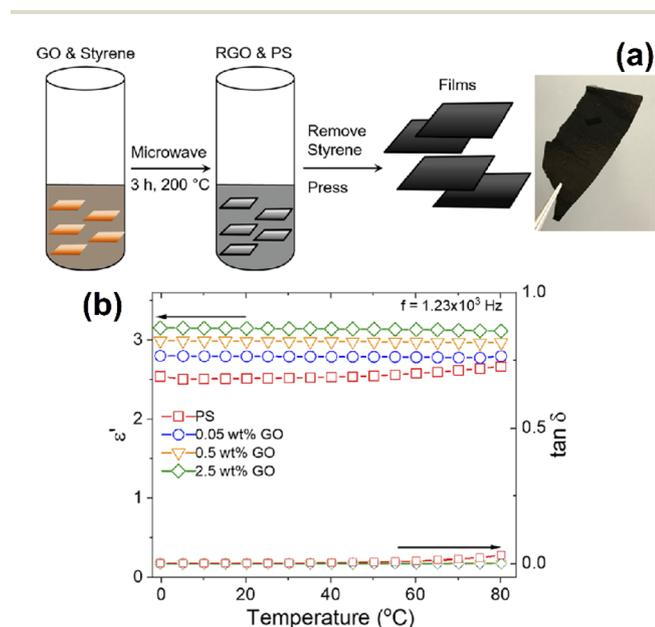
Fig. 16 (a) Overview of the synthetic and processing method for the preparation of RGO/PS polymer nanocomposites (b) temperature dependence on the static dielectric constant and  $\tan \delta$  of RGO/PS nanocomposite materials. Reproduced with permission from ref. 111. Copyright 2020 American Chemical Society.
