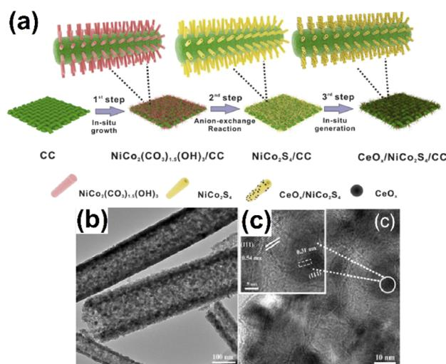
Fig. 15 (a) Schematic illustration of the formation of  $\text{CeO}_x/\text{NiCo}_2\text{S}_4/\text{CC}$ , (b) TEM images of  $\text{CeO}_x/\text{NiCo}_2\text{S}_4/\text{CC}$ , and (c) HRTEM image of  $\text{CeO}_x/\text{NiCo}_2\text{S}_4/\text{CC}$ . Reproduced with permission from ref. 98. Copyright 2019 American Chemical Society.
