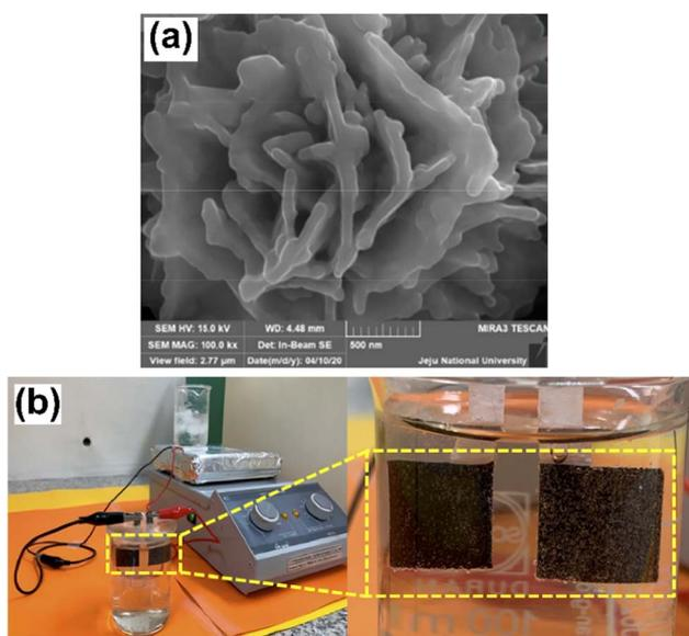
Fig. 7 (a) FE-SEM micrographs of the CuFeS<sub>2</sub> nanostructure obtained under various magnifications and (b) the real time application of thermoelectrically-driven self-powered water electrolyzer using CuFeS<sub>2</sub> as both the negative (cathode) and positive (anode) electrode in 1.0 M KOH electrolyte. Reproduced with permission from ref. 60. Copyright 2021 American Chemical Society.
