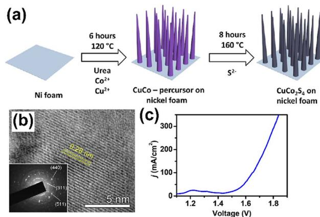
Fig. 6 (a) Schematic illustration of the formation of CuCo<sub>2</sub>S<sub>4</sub> nanowire arrays on nickel foam, (b) HR-TEM image of CuCo<sub>2</sub>S<sub>4</sub> with the SAED image in the inset, (c) the overall WS of CuCo<sub>2</sub>S<sub>4</sub>/NF//CuCo<sub>2</sub>S<sub>4</sub>/NF at a scan rate of  $5 \text{ mV s}^{-1}$ . Reproduced with permission from ref. 59. Copyright 2018 American Chemical Society.
