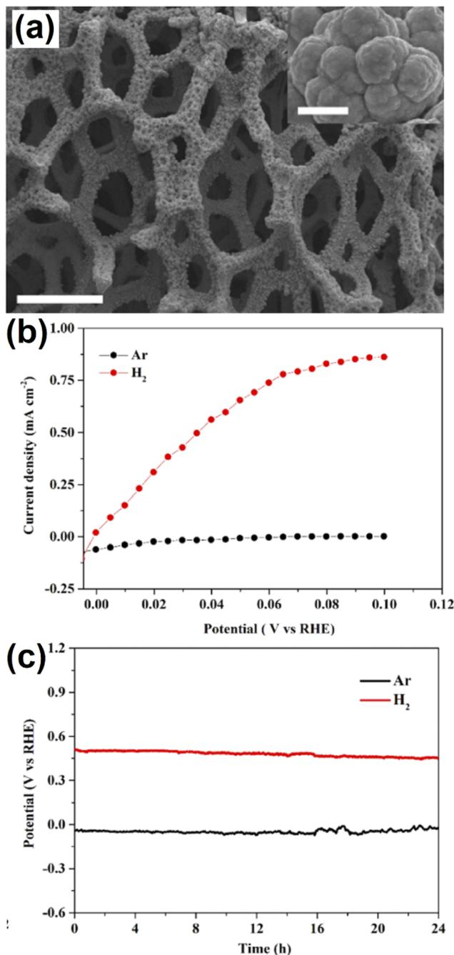
Fig. 3 (a) SEM image of B-Ni, (b) Steady-state polarization curves of B-Ni for the HOR in Ar- and H<sub>2</sub>-saturated 0.1 M KOH, and (c) Chronoamperometry curves of B-Ni in Ar- and H<sub>2</sub>-saturated 0.1 M KOH measured at 0.10 V versus RHE. Reproduced with permission from ref. 38. Copyright 2021 American Chemical Society.
