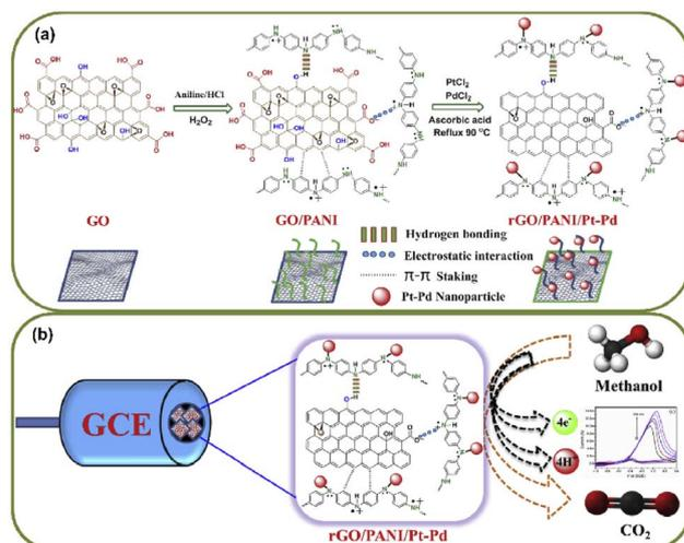
Fig. 12 Schematic illustration of (a) the preparation of rGO/PANI/Pt–Pd and (b) the electrocatalytic oxidation of methanol on rGO/PANI/Pt–Pd. Reproduced with permission from ref. 88. Copyright 2019 Elsevier Publications.
