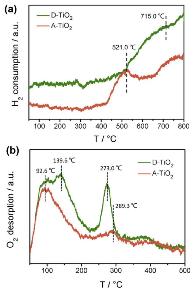
Fig. 10 (a) H<sub>2</sub>-TPR profiles of A-TiO<sub>2</sub> and D-TiO<sub>2</sub>, (b) O<sub>2</sub>-TPD profiles of A-TiO<sub>2</sub> and D-TiO<sub>2</sub>. Reproduced with permission from ref. 78. Copyright 2019 American Chemical Society.
