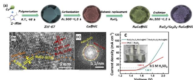
Fig. 14 (a) Schematic illustration of the synthesis process of  $\text{RuO}_2/\text{Co}_3\text{O}_4\text{-RuCo@NC}$ , (b) enlarged HRTEM images and FFT patterns in section I and section II, and (c) the polarization curves for overall WS in 0.5 M  $\text{H}_2\text{SO}_4$ . Reproduced with permission from ref. 97. Copyright 2019 American Chemical Society.
