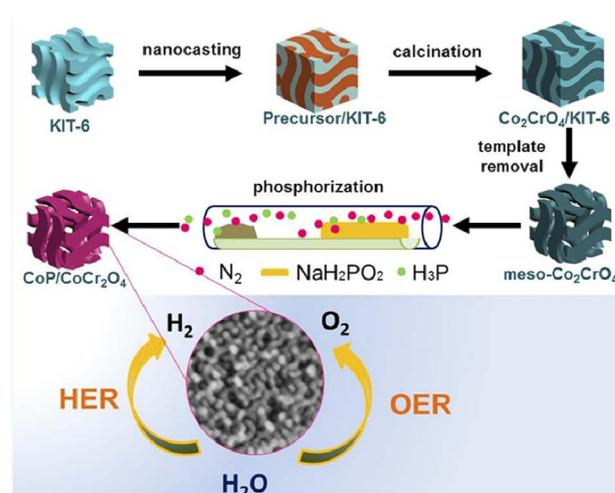
Fig. 2 Schematic illustration of the synthetic strategy of the meso-porous CoP/CoCr<sub>2</sub>O<sub>4</sub> heterojunction for the HER measured in 1.0 M KOH solution. Reproduced with permission from ref. 36. Copyright 2020 American Chemical Society.
