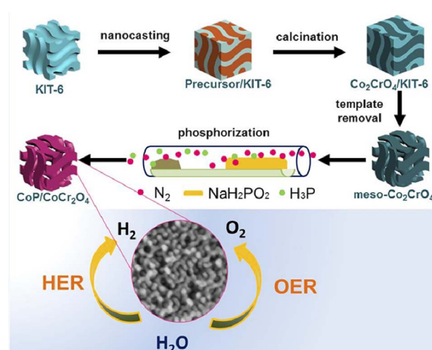
Fig. 2 Schematic illustration of the synthetic strategy of the meso-porous CoP/CoCr 2 O 4 heterojunction for the HER measured in 1.0 M KOH solution. Reproduced with permission from ref. 36. Copyright 2020 American Chemical Society.
