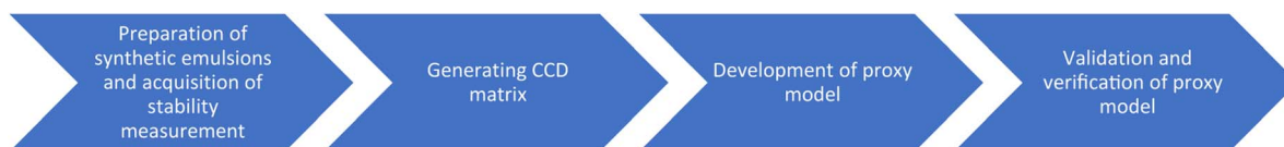
Fig. 1 Steps for developing a proxy model for the prediction of emulsion stability.
