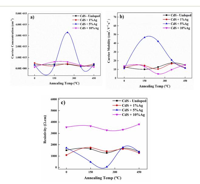
Fig. 8 The electrical properties of undoped CdS and Aq-doped CdS films; (a) carrier concentration, (b) carrier mobility, (c) resistivity.
