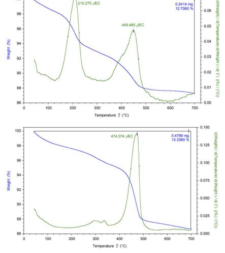
Fig. 5 TG/DTA analysis of CM@SS-BBTU (top) and CM@SS-BBTU-Cu(II) (bottom)
