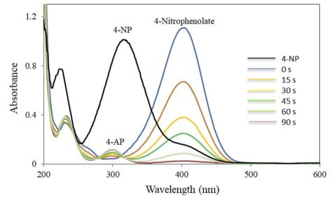
Fig. 7 UV-Vis spectra of the reduction of 4-NP in the presence of NaBH₄ and CM@SS-BBTU-Cu(II).
