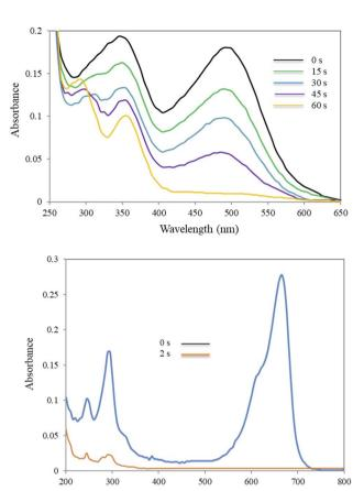
Fig. 8 Alterations in UV-Vis spectra of CR (top) and MB (bottom) with time in  $NaBH_4$ -mediated catalytic reduction.
