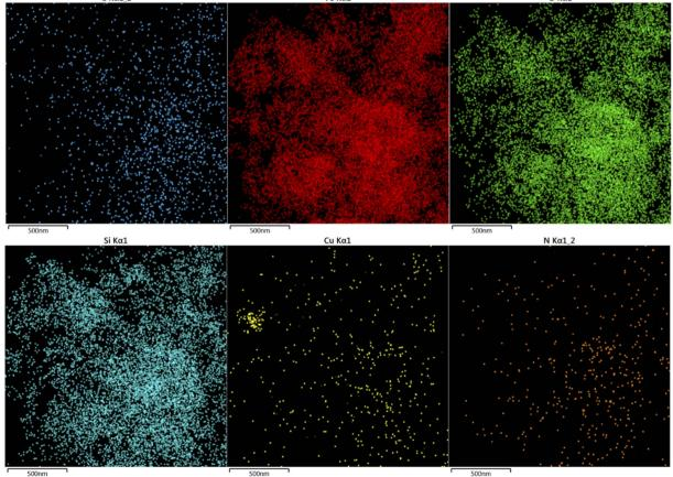
Fig. 2 EDS analysis and elemental mapping of CM@SS-BBTU-Cu(II).
