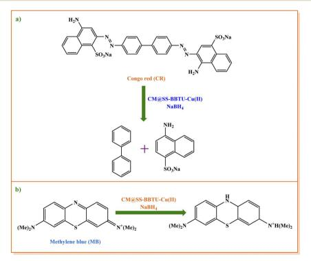
Scheme 4 CM@SS-BBTU-Cu(ii)-catalyzed reduction of (a) CR and (b) MB using NaBH<sub>4</sub>.
