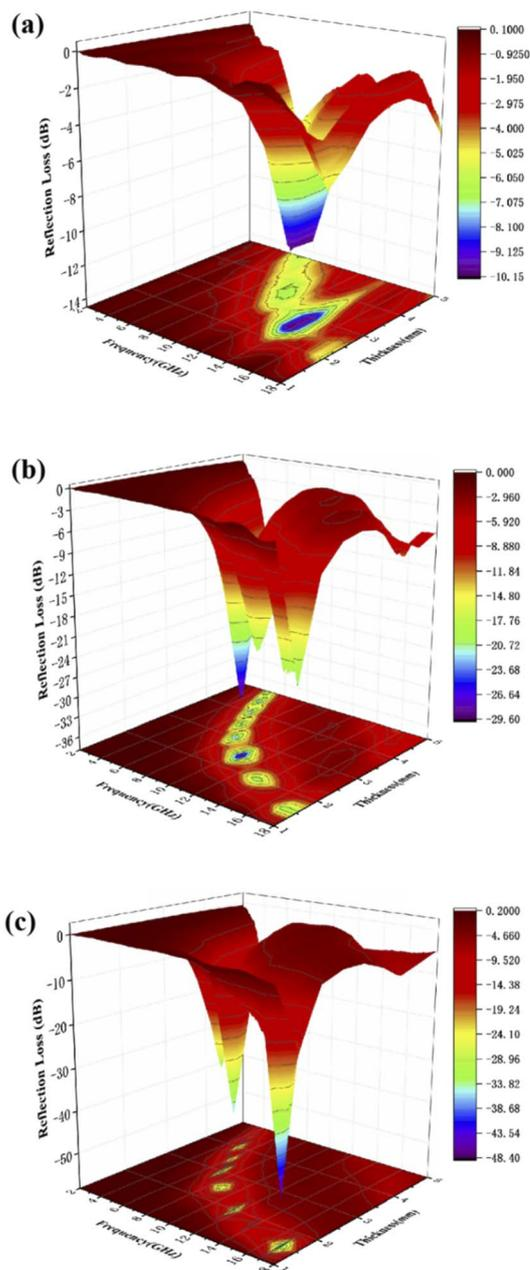
Fig. 7 Three-dimensional plots of reflection loss values for paraffin composites of cobalt sulfide with 30% filling ratio of C1 (a), 40% filling ratio of C1 (b) and 50% filling ratio of C1 (c).
