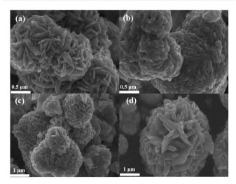
Fig. 2 (a) The SEM image of C1 after reacting at 200 °C, (b) the SEM image of C2 after reacting at 210  $^{\circ}\text{C}$  (c) the SEM image of C3 after reacting at 220 °C, the SEM image of C4 after reacting at 230 °C.
