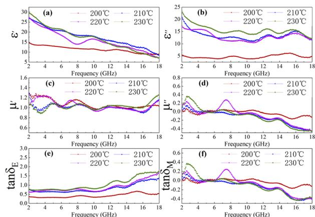
Fig. 4 The  $\epsilon'$  (a),  $\epsilon''$  (b),  $\mu'$  (c),  $\mu''$  (d), (e) dielectric loss tangent ( $\tan \delta_e = \epsilon''/\epsilon'$ ) and (f) magnetic loss tangent ( $\tan \delta_m = \mu''/\mu'$ ) of C1 to C4 paraffin composites with 50% filling ratio.
