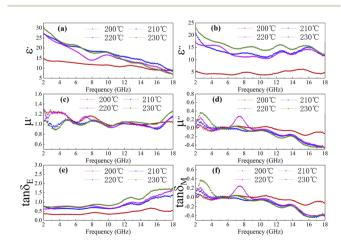
Fig. 4 The  $\varepsilon'$  (a),  $\varepsilon''$  (b),  $\mu'$  (c),  $\mu''$  (d), (e) dielectric loss tangent (tan  $\delta_{\rm e} =$  $\varepsilon''/\varepsilon'$ ) and (f) magnetic loss tangent (tan  $\delta_{\rm m}=\mu''/\mu'$ ) of C1 to C4 paraffin composites with 50% filling ratio.
