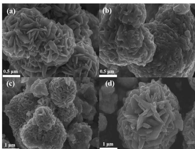
Fig. 2 (a) The SEM image of C1 after reacting at  $200\text{ }^\circ\text{C}$ , (b) the SEM image of C2 after reacting at  $210\text{ }^\circ\text{C}$  (c) the SEM image of C3 after reacting at  $220\text{ }^\circ\text{C}$ , the SEM image of C4 after reacting at  $230\text{ }^\circ\text{C}$ .
