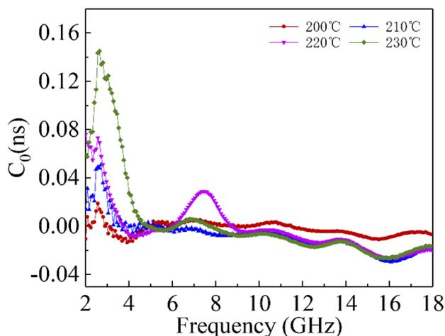
Fig. 6 Constant  $C_0$  of cobalt sulfide with 50% filling ratio under different reaction temperature.
