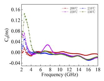
Fig. 6 Constant  $C_0$  of cobalt sulfide with 50% filling ratio under diffierent reaction temperature.
