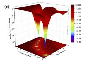
Fig. 7 Three-dimensional plots of reflection loss values for paraffin composites of cobalt sulfide with 30% filling ratio of C1 (a), 40% filling ratio of C1 (b) and 50% filling ratio of C1 (c).
