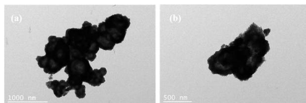
Fig. 3 (a) and (b) The TEM image of CoS under different resolutions.
