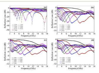
Fig. 8 Reflection loss at different temperature and thicknesses for cobalt sulfide composites of C1 (a), C2 (b), C3 (c) and C4 (d) with filling ratios of 50%.
