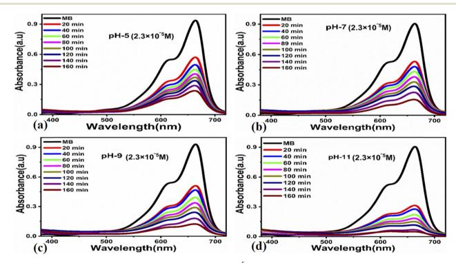
Fig. 5 UV-visible absorbance spectra at an MB concentration of  $2.3 \times 10^{-5}$  M at different pH values of the dye solution for the time interval of 160 min under the irradiation of UV light using a catalyst dose of 15 mg (a) pH 5, (b) pH 7, (c) pH 9, (d) pH 11.
