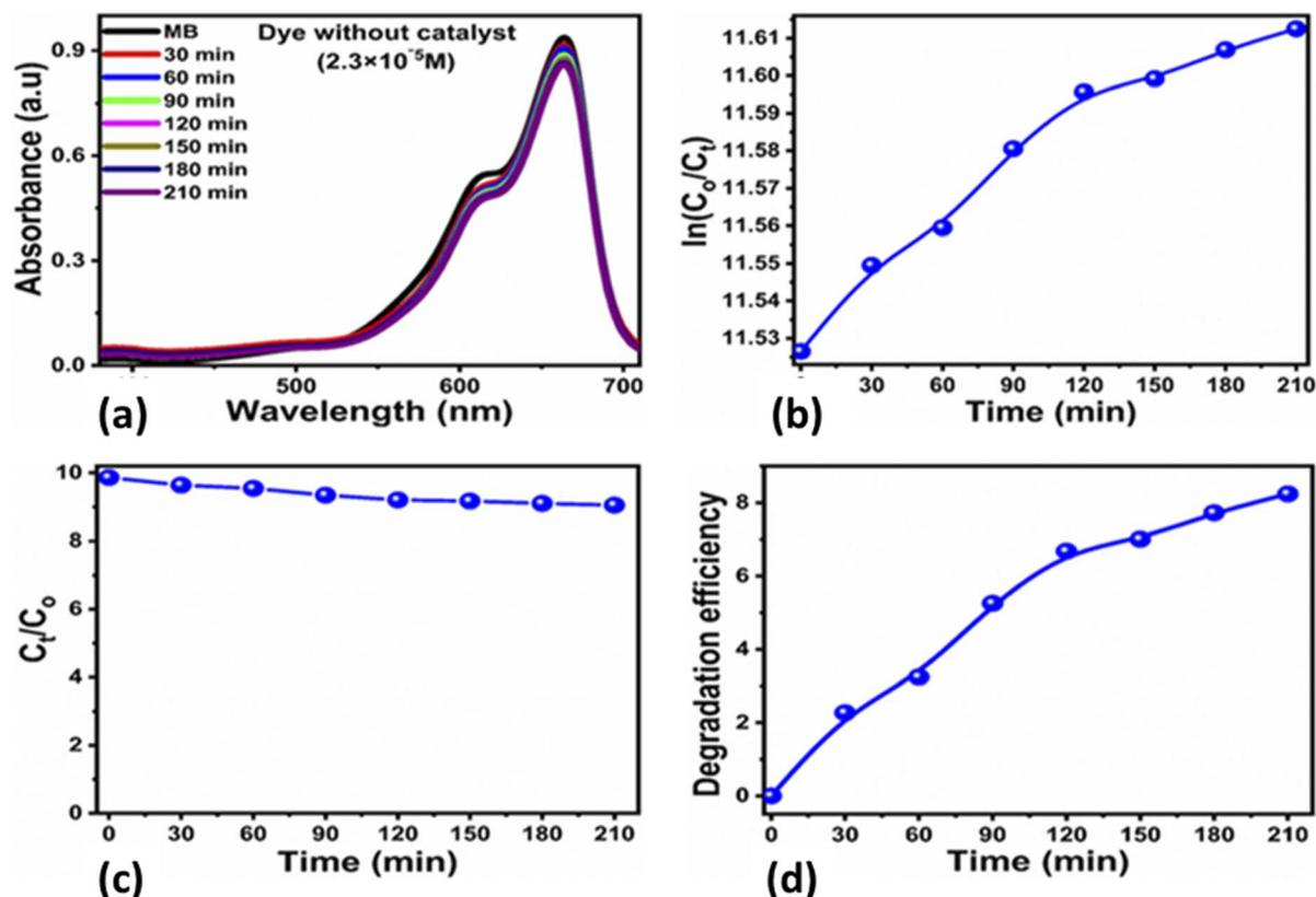
Fig. 9 (a) UV-visible absorbance spectra of the MB concentration of  $2.3 \times 10^{-5}$  M without the use of the photocatalyst for the time interval of 210 min under the irradiation of UV light, (b, c) reaction kinetics with the photocatalyst, (d) degradation efficiency without the photocatalyst.
