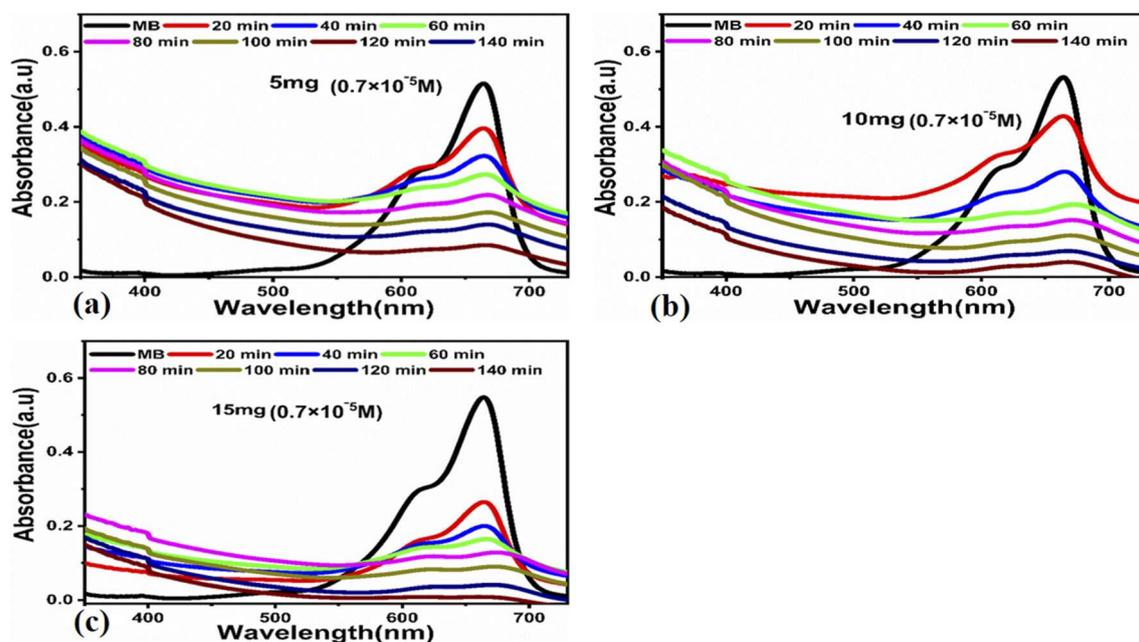
Fig. 3 UV-visible absorbance spectra at an MB concentration of  $0.7 \times 10^{-5}$  M for the time interval of 140 min under the irradiation of UV light (a) a catalyst dose of 5 mg, (b) a catalyst dose of 5 mg, (c) a catalyst dose of 5 mg.
