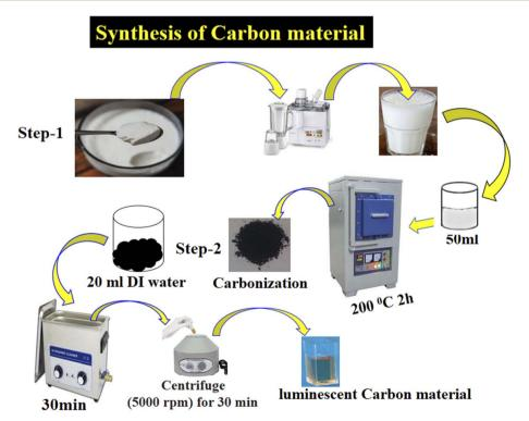
Scheme 1 Scheme of the green and innovative carbon material synthesis process.
