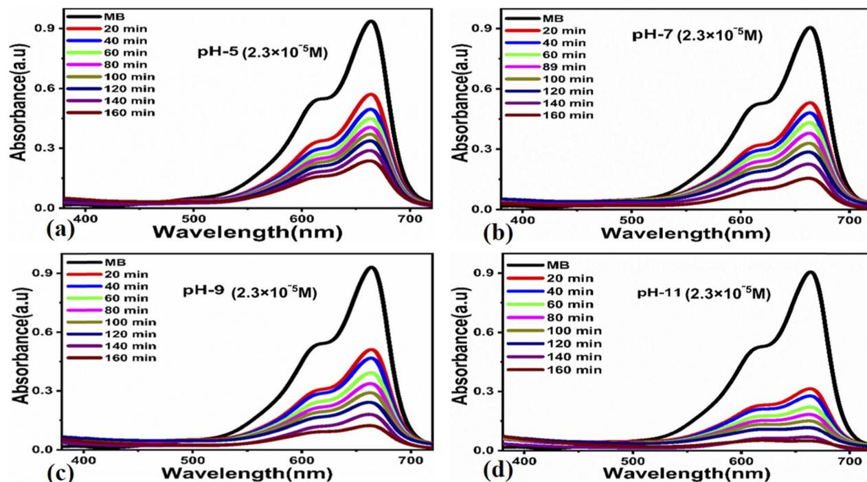
Fig. 5 UV-visible absorbance spectra at an MB concentration of  $2.3 \times 10^{-5}$  M at different pH values of the dye solution for the time interval of 160 min under the irradiation of UV light using a catalyst dose of 15 mg (a) pH 5, (b) pH 7, (c) pH 9, (d) pH 11.
