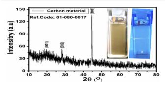
Fig. 2 XRD diffraction patterns of the carbon material obtained from yogurt; the inset shows the luminescent aspects of the carbon material.
