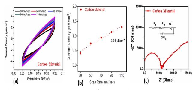
Fig. 11 (a) Cyclic voltammetry curves at various scan rates in  $2.3 \times 10^{-5}$  M solution of MB, (b) linear fitting of the current density at various scan rates, (c) EIS spectrum of the as-prepared carbon material in  $2.3 \times 10^{-5}$  M solution of MB.
