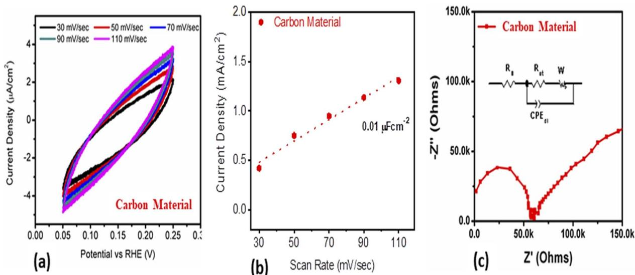
Fig. 11 (a) Cyclic voltammograms at various scan rates in  $2.3 \times 10^{-5}$  M solution of MB, (b) linear fitting of the current density at various scan rates, (c) EIS spectrum of the as-prepared carbon material in  $2.3 \times 10^{-5}$  M solution of MB.
