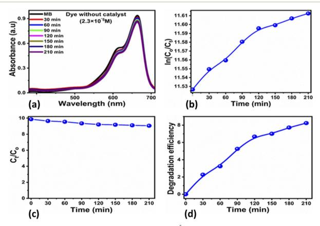
Fig. 9 (a) UV-visible absorbance spectra of the MB concentration of  $2.3 \times 10^{-5}$  M without the use of the photocatalyst for the time interval of 210 min under the irradiation of UV light, (b, c) reaction kinetics with the photocatalyst, (d) degradation efficiency without the photocatalyst.
