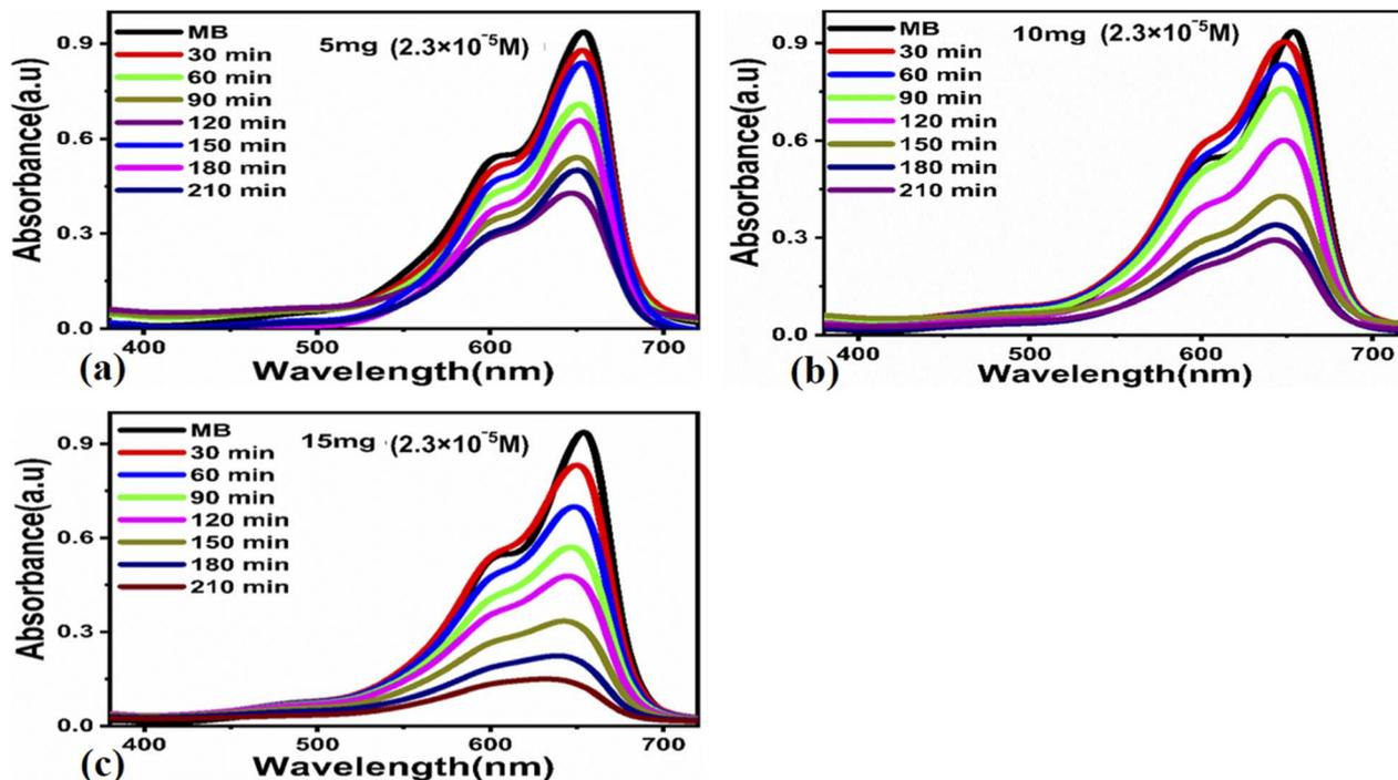
Fig. 4 UV-visible absorbance spectra at an MB concentration of  $2.3 \times 10^{-5}$  M for the time interval of 210 min under the irradiation of UV light (a) a catalyst dose of 5 mg, (b) a catalyst dose of 10 mg, (c) a catalyst dose of 15 mg.
