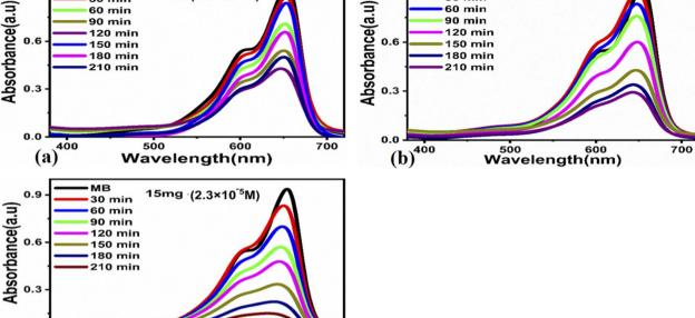
Fig. 4 UV-visible absorbance spectra at an MB concentration of  $2.3 \times 10^{-5}$  M for the time interval of 210 min under the irradiation of UV light (a) a catalyst dose of 5 mg, (b) a catalyst dose of 10 mg, (c) a catalyst dose of 15 mg
