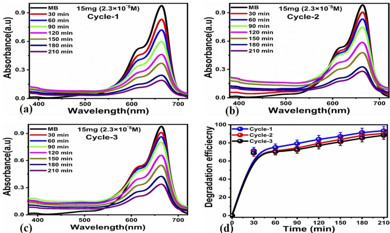
Fig. 10 UV-visible absorbance spectra at an MB concentration of  $2.3 \times 10^{-5}$  M for understanding the reusability of the carbon material for a time interval of 160 min under the irradiation of UV light using a catalyst dose of 15 mg (a) cycle-1, (b) cycle-2, (c) cycle-3, (d) % photodegradation efficiency.
