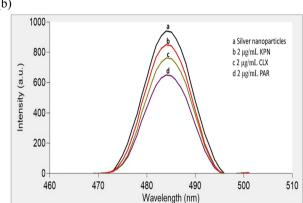
Fig. 3 (a) FL excitation and emission spectra of blank and SNPs at 242/485 nm, where (a and a\*) are spectra for blank and (b and b\*) are for SNPs. (b) FL emission spectra of (a) SNPs and (b, c, d) in the presence of KPN, CLX and PAR 2  $\mu$ g mL<sup>-1</sup> each, respectively at 484 nm.
