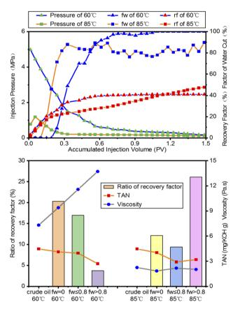
Fig. 2 Injection pressure, factor of the water cut  $(f_{\rm w})$  and recovery factor  $(r_{\rm f})$  as functions of the accumulated injection volume in the water flooding experiments (top). Comparison of the ratio of the recovery factor, viscosity and total acid number (TAN) values of the crude oil and produced oils from different water flooding stages (bottom).
