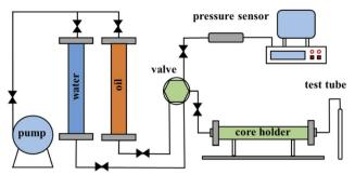
Fig. 1 Schematic diagram of the water flooding experiment instrument.
