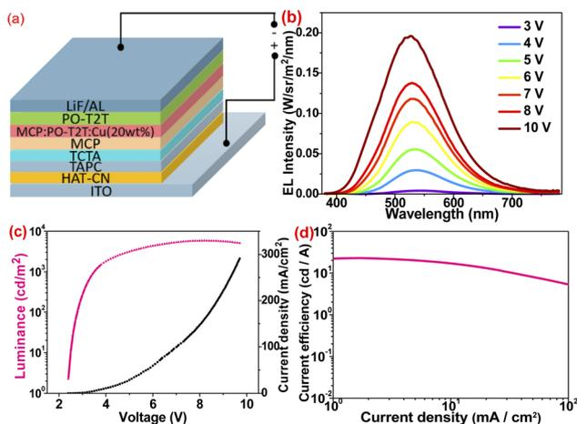
Fig. 8 (a) The OLED device structure of **2**-based device; (b) the EL spectra of 20 wt% doping device under different voltages of **2**; (c) current density–voltage–brightness ( $I$ – $V$ – $B$ ) curves of **2**-based device; (d) the dependence of the current efficiency of **2** on the current density.
