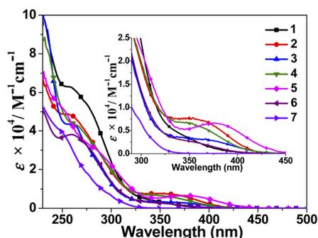
Fig. 4 The UV/vis spectra of 1–7 in CH<sub>2</sub>Cl<sub>2</sub> solution.
