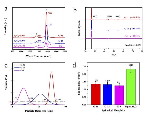
Fig. 3 Three kinds of spherical graphite: (a) Raman spectra, (b) wide-angle XRD patterns, (c) particle size distribution curves, (d) tap density.
