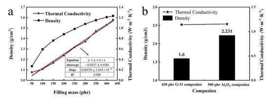
Fig. 4 (a) The density and thermal conductivity of G-31 filled composite under different filling contents, (b) the density relationships of the two composites under the same thermal conductivity.
