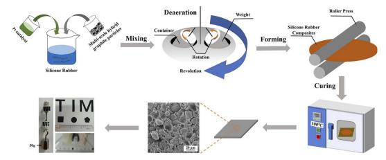
Fig. 1 Preparation processes of the spherical graphite composites.
