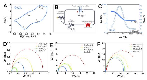
Fig. 5 (A): Voltammetric profile of the  $Co_3O_4$  in 0.1 M  $Na_2SO_4$  pH 7 with a scan rate at 50 mV s<sup>-1</sup>; (B): electrical equivalent circuit derived from Nyquist plots; (C): Bode plot for  $Co_3O_4$  in 0.1 M  $Na_2SO_4$  pH 7; Nyquist plots derived from EIS measurements of the catalysts films at: 0.1 mol  $L^{-1}$  HNO<sub>3</sub> pH 1 (D); 0.1 mol  $L^{-1}$  Na<sub>2</sub>SO<sub>4</sub> pH 7 (E); 0.1 mol  $L^{-1}$  NaOH pH 13 (F), at a scan rate of 5 mV s<sup>-1</sup>.
