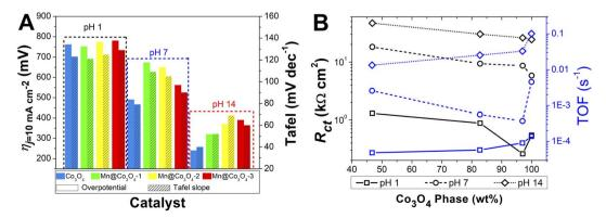
Fig. 7 (A): Histograms of the required overpotentials at 10 mA cm<sup>-2</sup> and Tafel slopes for all pHs. (B): Correlation of  $R_{ct}$  and TOF with the percentage of  $Co_3O_4$  phase.
