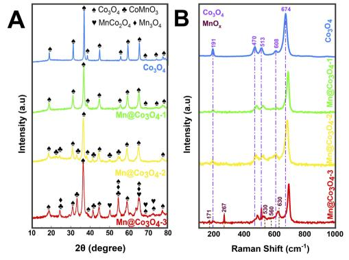
Fig. 1 (A) Powder X-ray diffraction patterns, and (B) Raman spectra of the Mn-doped Co<sub>3</sub>O<sub>4</sub>.
