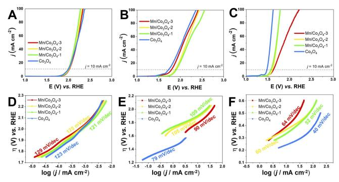
Fig. 6 Polarization LSV curves for oxygen evolution reactions of the catalysts films RDE electrode. (A): pH 1, (B): pH 7, (C): pH 14; and respective Tafel plots: (D): pH 1, (E): pH 7, (F): pH 14, at a scan rate of 0.005 V s<sup>-1</sup>.
