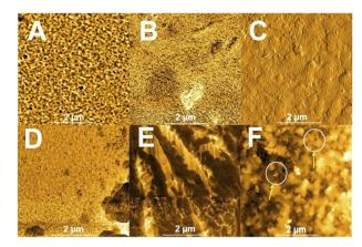
Fig. 4 AFM images of  $\partial C/\partial z$  of the catalysts films. (A): FTO, (B): Mn@Co<sub>3</sub>O<sub>4</sub>-3, (C): Mn@Co<sub>3</sub>O<sub>4</sub>-2, (D): Mn@Co<sub>3</sub>O<sub>4</sub>-1, (E): Co<sub>3</sub>O<sub>4</sub>, (F): zoom Mn@Co<sub>3</sub>O<sub>4</sub>-2 areas.
