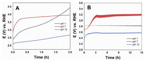
Fig. 8 Long-term stability electrolysis in  $Co_3O_4$  on (A) FTO (j=10 mA cm $^{-2}$ ) and (B) RDE (j=141 mA cm $^{-2}$ ) under a constant current of 10 mA in 0.1 mol L $^{-1}$  HNO $_3$  pH 1, 0.1 mol L $^{-1}$  Na $_2$ SO $_4$  pH 7, and 0.1 mol L $^{-1}$  NaOH pH 13.
