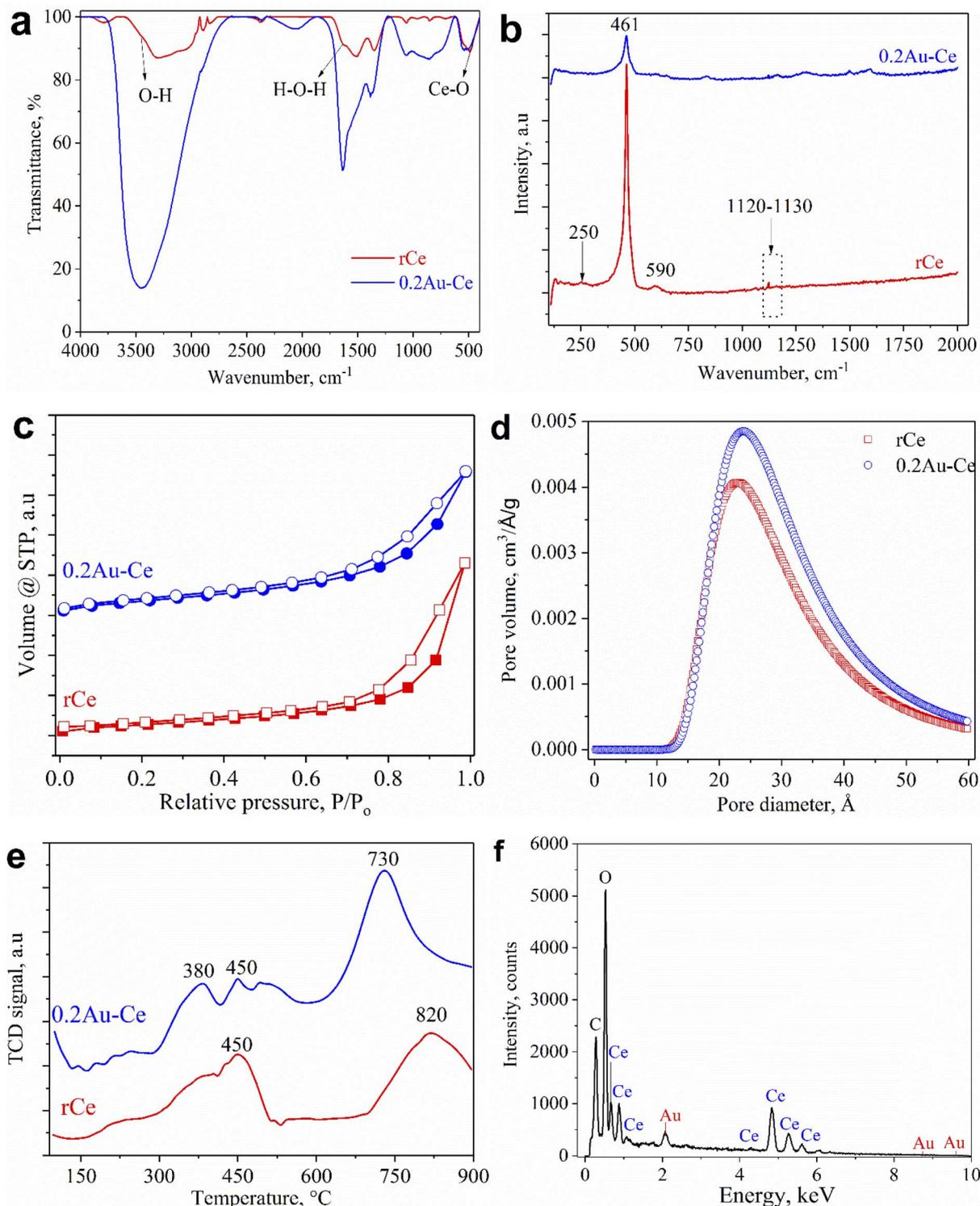
Fig. 2 FT-IR (a) and Raman (b) spectra, N<sub>2</sub> adsorption/desorption isotherms (c), BJH pore diameter distributions (d), H<sub>2</sub>-TPR patterns (e), and EDS spectrum (f) of samples.
