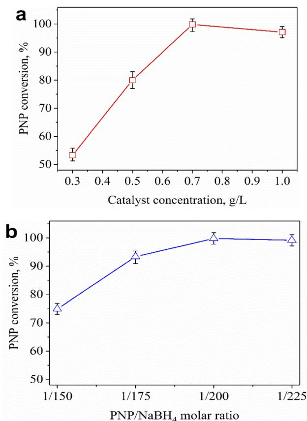
Fig. 6 Effect of catalyst concentration (a) and PNP/NaBH<sub>4</sub> molar ratio (b) on the catalytic activity of 0.2Au–Ce sample after 30 min.
