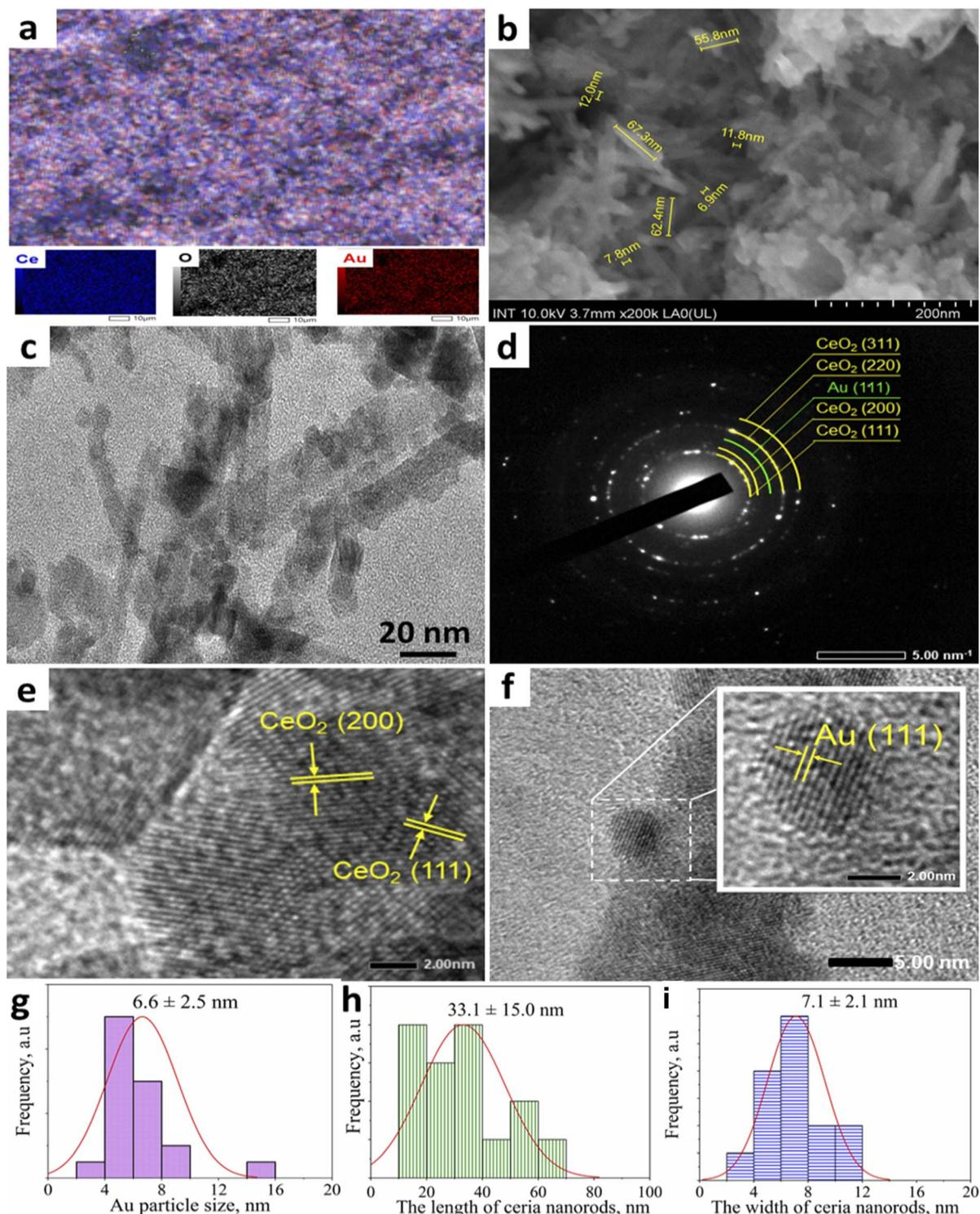
Fig. 4 Element mapping (a), FESEM (b), HRTEM (c), SAED (d), CeO<sub>2</sub> and Au, planes (e, f) images, and the size distribution histograms of Au nanoparticles (g) and length (h), width (i) of ceria nanorods of 0.2Au–Ce sample.
