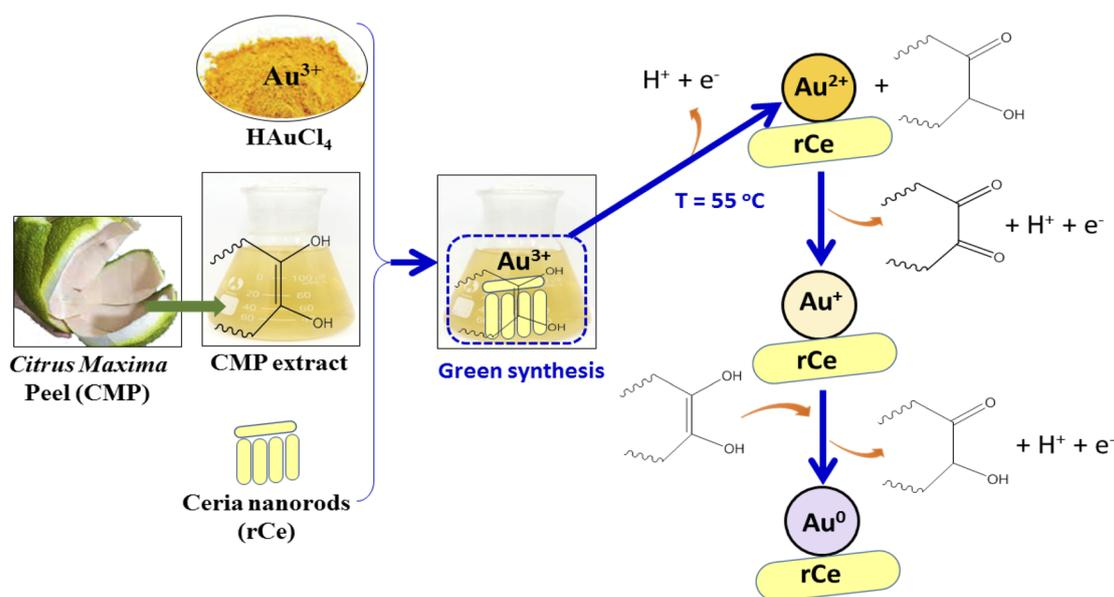
Fig. 3 The mechanism to form green-synthesized gold nanoparticles (Au<sup>0</sup>) decorated on ceria nanorods (r-Ce).
