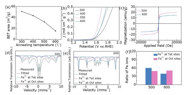
Fig. 4 (a) BET surface area of all samples, (b) BET surface area normalized LSV plot, (c) magnetic hysteresis loops, (d) Mössbauer spectra of 500, and (e) 600 at room temperature. (f) The ratio of Fe ions in different sites for 500 and 600.
