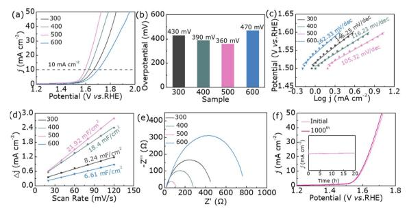
Fig. 3 (a) OER LSV curves, (b)  $\eta$ 10 and (c) Tafel plots of 300, 400, 500, and 600 for the OER. (d) Double-layer capacitance plots ( $C_{cl}$ ) and (e) Nyquist plots of 300, 400, 500, and 600. (f) LSV curves of the sample 500 catalyst before and after 1000 cycles; inset is its chronoamperometry test.
