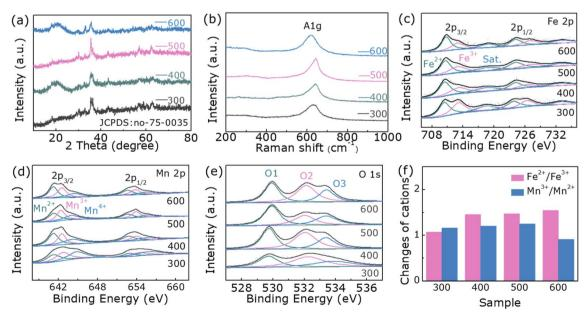
Fig. 1 (a) X-ray diffraction patterns, (b) Raman spectrum, (c) Fe 2p spectrum, (d) Mn 2p spectrum and (e) O 1s spectrum of sample 300, 400, 500 and 600. (f) Relative strength of different valence cations.
