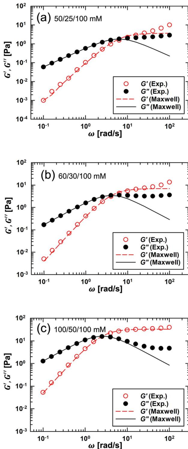
Fig. 4 Shear storage ( $G'$ ) and loss ( $G''$ ) moduli as functions of angular frequency ( $\text{rad s}^{-1}$ ) for three different WLM solutions: (a) 50/25/100, (b) 60/30/100, (c) 100/50/100 mM (CPyCl/NaSal/NaCl).
