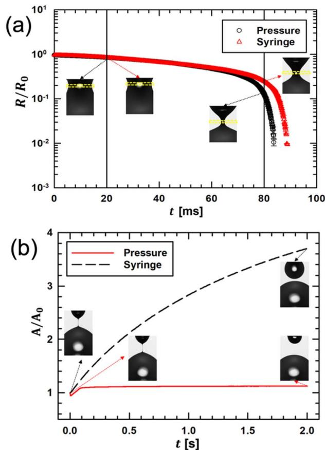
Fig. 2 (a) Capillary-thinning and pinch-off dynamics of 95% glycerin solution when flow rate from nozzle to the substrate is controlled by syringe pump and stop-flow system.  $R_0$  denotes outer radius of nozzle. (b) change in size of droplet hanging from nozzle tip following pinch-off. Time-dependent droplet size ( $A$ ) is normalized to its initial size ( $A_0$ ) immediately prior to pinch-off.
