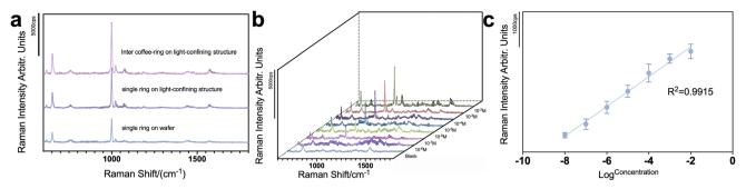
Fig. 5 (a) Raman spectra of  $10^{-2}$  M TPhT using the inter-coffee-ring on the light-confining structure, a single coffee-ring on the light-confining structure, and a single coffee-ring on a wafer (laser power set to 7 mW), (b) SERS detection of TPhT spiked tap water with different concentrations, and (c) the linear regression of signal intensities at 995 cm<sup>-1</sup> plot against log concentrations.
