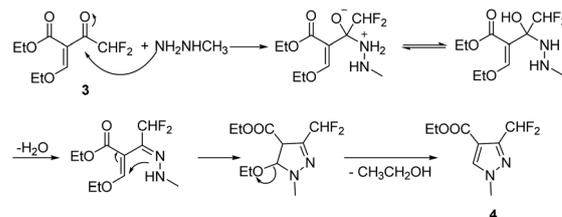
Scheme 2 Synthetic mechanism of the intermediate 4.
