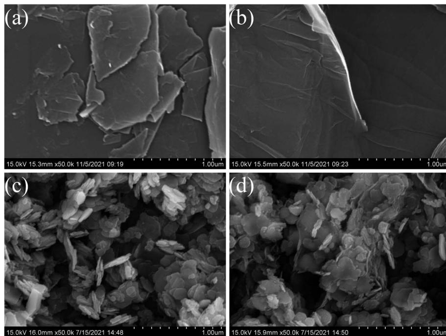
Fig. 1 SEM images of (a) graphite, (b) GO, (c) fresh RGO/Fe<sub>3</sub>O<sub>4</sub> (RGO/Fe<sub>3</sub>O<sub>4</sub>-2) and (d) used RGO/Fe<sub>3</sub>O<sub>4</sub> (RGO/Fe<sub>3</sub>O<sub>4</sub>-2,  $C_0 = 135.88 \text{ mg L}^{-1}$ ,  $T = 298 \text{ K}$ ,  $m = 0.050 \text{ g}$ ,  $t = 180 \text{ min}$ ,  $\text{pH} = 11.74$ ).
