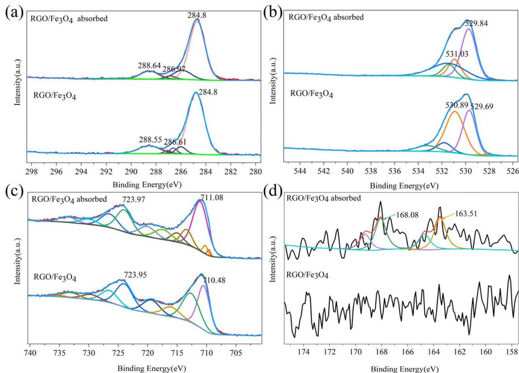
Fig. 3 XPS spectra of (a) C 1s, (b) O 1s, (c) Fe 2p and (d) S 2p of fresh and used RGO/Fe<sub>3</sub>O<sub>4</sub> (RGO/Fe<sub>3</sub>O<sub>4</sub>-2,  $C_0 = 135.88 \text{ mg L}^{-1}$ ,  $T = 298 \text{ K}$ ,  $m = 0.050 \text{ g}$ ,  $t = 180 \text{ min}$ ,  $\text{pH} = 11.74$ ).
