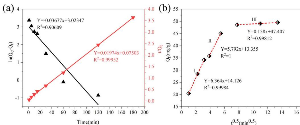
Fig. 7 Linear plots of (a) PFO and PSO models, and (b) IPD model ( $C_0 = 133.10 \text{ mg L}^{-1}$ ,  $T = 298 \text{ K}$ ,  $m = 25 \text{ mg}$ ,  $\text{pH} = 11.72$ ).
