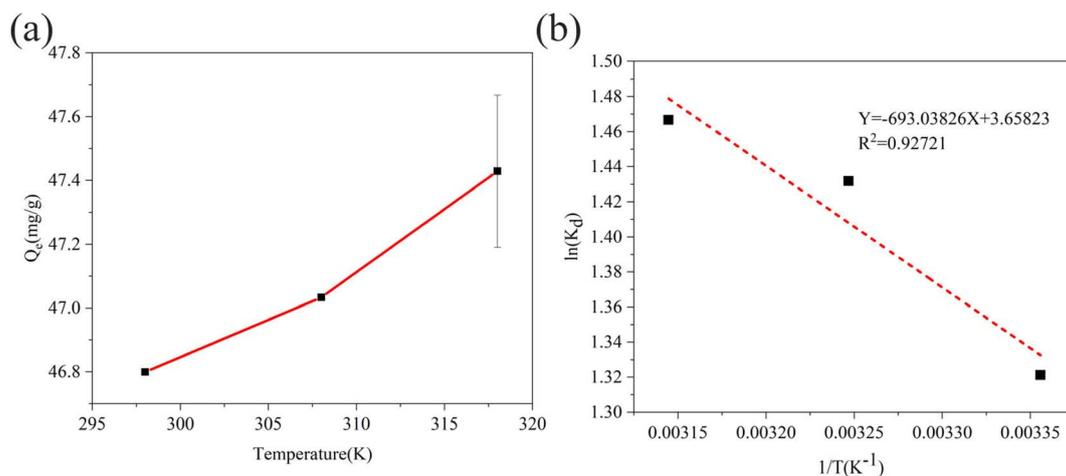
Fig. 9 (a) Effect of temperature on sulfide adsorption using RGO/Fe<sub>3</sub>O<sub>4</sub> ( $C_0 = 130.23 \text{ mg L}^{-1}$ ,  $m = 25 \text{ mg}$ ,  $t = 180 \text{ min}$ ,  $\text{pH} = 11.72$ ). Error bars represent the standard deviation of replicate measurements. (b) The plot of  $\ln(K_d)$  vs.  $1/T$  for the sulfide adsorption on RGO/Fe<sub>3</sub>O<sub>4</sub>.
