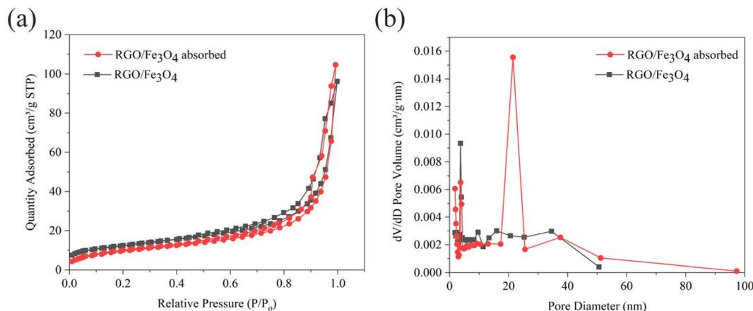
Fig. 4 (a) N<sub>2</sub> adsorption–desorption isotherms, and (b) pore size distribution of fresh and used RGO/Fe<sub>3</sub>O<sub>4</sub> (RGO/Fe<sub>3</sub>O<sub>4</sub>-2,  $C_0 = 119.31 \text{ mg L}^{-1}$ ,  $T = 298 \text{ K}$ ,  $m = 0.4 \text{ g}$ ,  $t = 180 \text{ min}$ ,  $\text{pH} = 11.70$ ).
