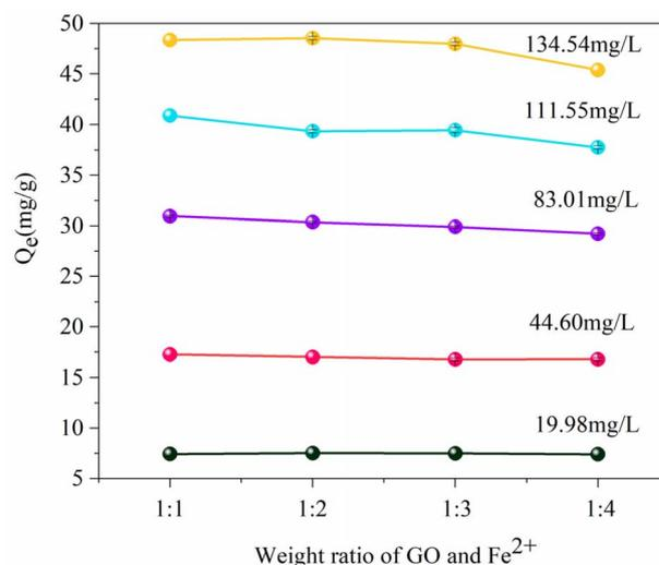
Fig. 5 The sorption capacities of various RGO/Fe<sub>3</sub>O<sub>4</sub> ( $T = 298$  K,  $m = 25$  mg,  $t = 180$  min). Error bars represent the standard deviation of replicate measurements.
