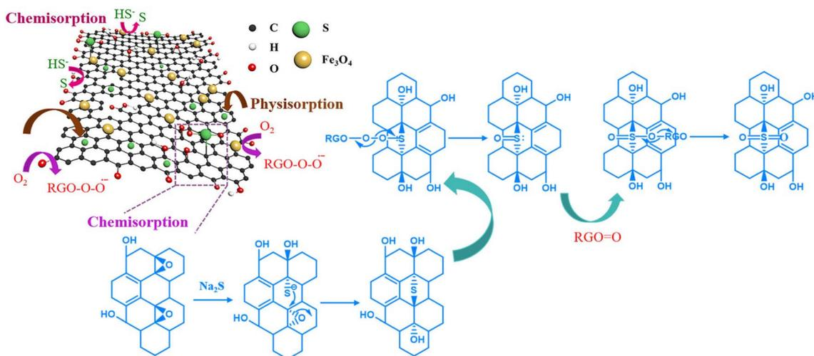
Fig. 10 Potential mechanism of sulfide removal by the RGO/Fe<sub>3</sub>O<sub>4</sub> hybrid material.
