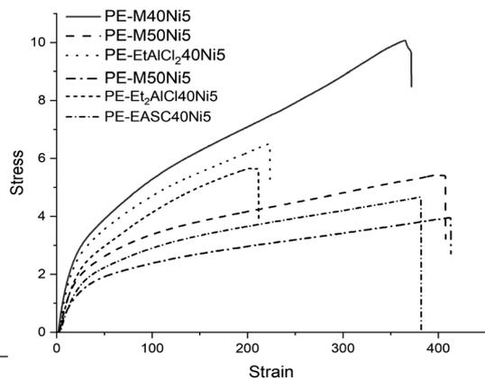
Fig. 5 Stress–strain curves for samples, PE-EtAlCl<sub>2</sub>40Ni<sub>5</sub>, PE-EtAlCl<sub>2</sub>50Ni<sub>5</sub>, PE-M40Ni<sub>5</sub>, PE-M50Ni<sub>5</sub>, PE-Et<sub>2</sub>AlCl<sub>40</sub>Ni<sub>5</sub> and PE-EASC40Ni<sub>5</sub>; the vertical line represents the breakage point.
