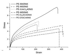
Fig. 5 Stress—strain curves for samples, PE-EtAlCl $_2$ 40Ni5, PE-EtAlCl $_2$ 50Ni5, PE-M40Ni5, PE-M50Ni5, PE-Et $_2$ AlCl40Ni5 and PE-EASC40Ni5; the vertical line represents the breakage point.
