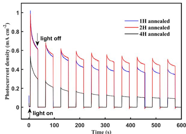
Fig. 5 Photocurrent density vs. time curves of the annealing WO<sub>3</sub> nanoflakes at 0.63 V vs. Ag/AgCl bias in the Na<sub>2</sub>SO<sub>4</sub> solution under AM 1.5 G illumination at room temperature.
