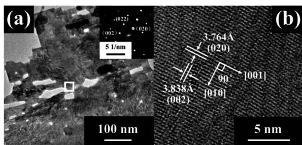
Fig. 3 (a) Low-magnification TEM image of the 2 H-WO<sub>3</sub> nanoflake (the inset shows the corresponding SAED pattern). (b) HRTEM images of the 2 H-WO<sub>3</sub> nanoflake taken from the area marked by a white square in (a).
