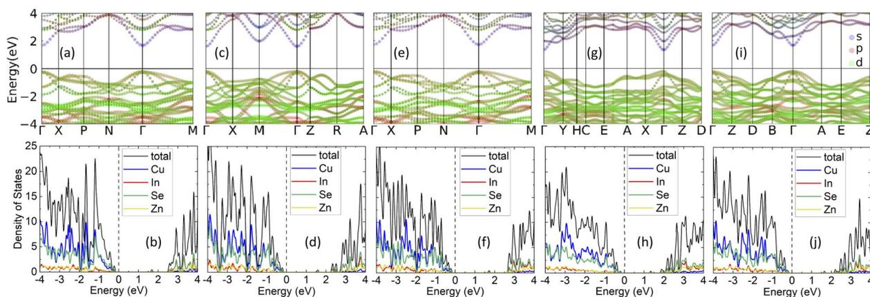
Fig. 2 Orbitaly projected band structure and atom projected density of states of the  $\text{CuZn}_2\text{InSe}_4$  phases: (a) and (b) KS; (c) and (d) PMCA; (e) and (f) ST; (g) and (h) WKS, and (i) and (j) WST. All results are obtained using the HSE06 hybrid functional.
