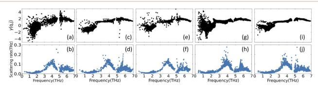
Fig. 5 Mode Grüneisen parameters  $\gamma(q, j)$  and room-temperature phonon scattering rates of (a) and (b) KS; (c) and (d) PMCA; (e) and (f) ST; (g) and (h) WKS and (i) and (j) WST of CuZn<sub>2</sub>InSe<sub>4</sub>.
