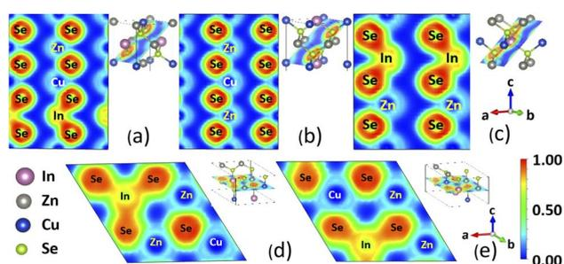
**Fig. 3** Electron localization function for (a) KS, (b) PMCA, (c) ST, (d) WKS, and (e) WST phases of  $\text{CuZn}_2\text{InSe}_4$  compounds. The different projections are shown at the right top corner next to each panel. The atomic composition and the ELF color scale are also displayed.
