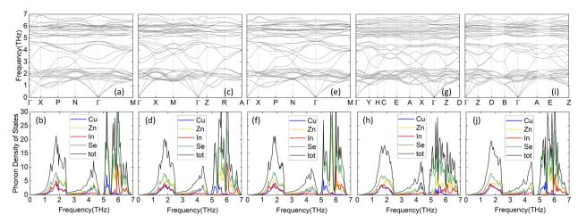
Fig. 4 Phonon dispersions and atomically resolved phonon density of states for the considered CuZn<sub>2</sub>InSe<sub>4</sub> phases for CuZn<sub>2</sub>InSe<sub>4</sub>: (a) and (b) KS; (c) (d) PMCA; (e) and (f) ST; (g) and (h) WKS, and (i) and (j) WST.
