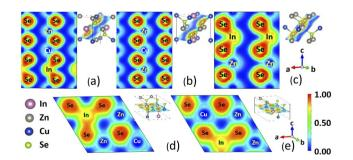
Fig. 3 Electron localization function for (a) KS, (b) PMCA, (c) ST, (d) WKS, and (e) WST phases of  $CuZn_2InSe_4$  compounds. The different projections are shown at the right top corner next to each panel. The atomic composition and the ELF color scale are also displayed.
