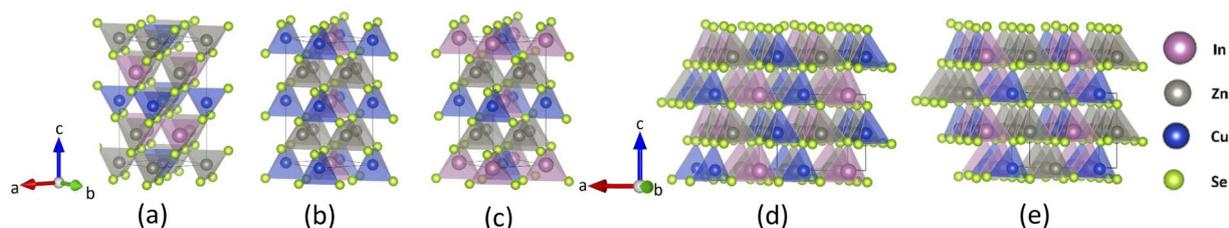
Fig. 1 Crystal structures for CuZn<sub>2</sub>InSe<sub>4</sub> with (a) kesterite (KS), (b) primitive mixed CuAu (PMCA), (c) stannite (ST), (d) wurtzite-kesterite (WKS), (e) wurtzite-stannite (WST) phases.
