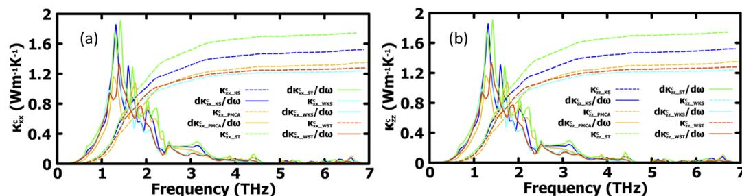
Fig. 7 Cumulative lattice thermal conductivity components and the first derivatives as a function of phonon frequency at 300 K along the (a) x-axis and (b) z-axis for the lattice phases of  $\text{CuZn}_2\text{InSe}_4$ .
