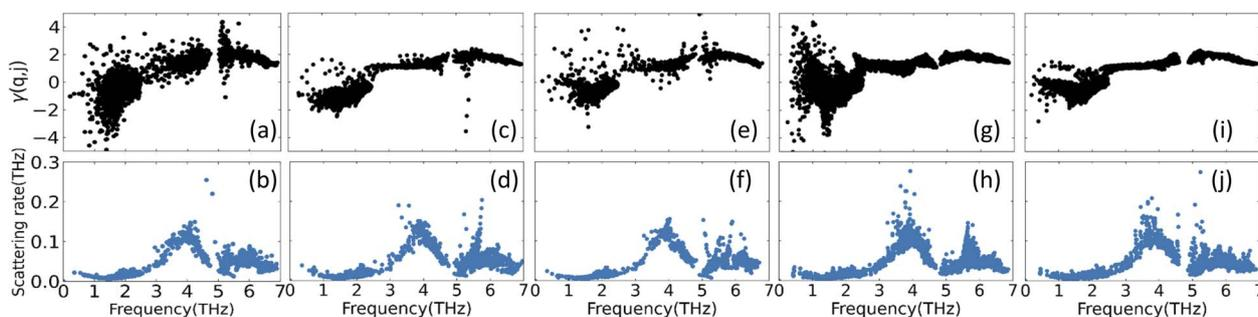
Fig. 5 Mode Grüneisen parameters  $\gamma(\mathbf{q}, j)$  and room-temperature phonon scattering rates of (a) and (b) KS; (c) and (d) PMCA; (e) and (f) ST; (g) and (h) WKS and (i) and (j) WST of  $\text{CuZn}_2\text{InSe}_4$ .
