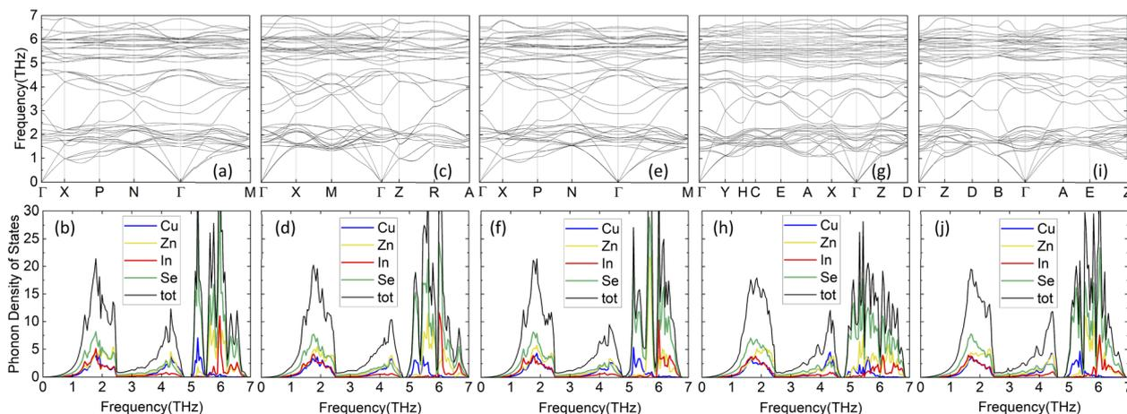
Fig. 4 Phonon dispersions and atomically resolved phonon density of states for the considered  $\text{CuZn}_2\text{InSe}_4$  phases for  $\text{CuZn}_2\text{InSe}_4$ : (a) and (b) KS; (c) (d) PMCA; (e) and (f) ST; (g) and (h) WKS, and (i) and (j) WST.
