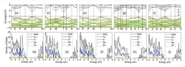
Fig. 2 Orbitally projected band structure and atom projected density of states of the CuZn₂InSe₄ phases: (a) and (b) KS; (c) and (d) PMCA; (e) and (f) ST; (g) and (h) WKS, and (i) and (j) WST. All results are obtained using the HSE06 hybrid functional.
