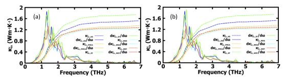
Fig. 7 Cumulative lattice thermal conductivity components and the first derivatives as a function of phonon frequency at 300 K along the (a) x-axis and (b) z-axis for the lattice phases of  $CuZn_2InSe_4$ .
