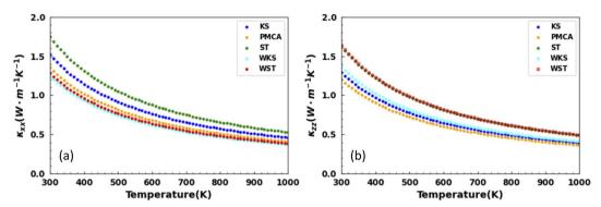
Fig. 6 Lattice thermal conductivity components as a function of temperature along the (a) x-axis and (b) z-axis for the lattice phases of  $CuZn_2InSe_4$ .
