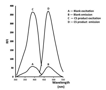
Fig. 3 Excitation and emission spectra of colistin (2  $\mu g$  mL $^{-1}$ ) with fluorogenic reagents.
