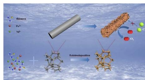
Fig. 1 Schematic of fabrication of Ni<sub>x</sub>Fe<sub>x</sub>S/NF-z M composite catalysts.
