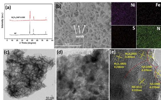
Fig. 2 (a) XRD patterns of the samples, (b) SEM images and the corresponding mapping of  $\text{Ni}_6\text{Fe}_2\text{S}/\text{NF}-0.05 \text{ M}$  collected on SEM, (c and d) TEM images and (e) HR-TEM image of  $\text{Ni}_6\text{Fe}_2\text{S}/\text{NF}-0.05 \text{ M}$ .
