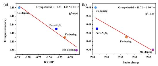
Fig. 5 The overpotential as a function of (a) ICOHP values of the active site Ni and HO\* intermediate and (b) bader charge of the active site for Ni<sub>3</sub>S<sub>2</sub>, and TM-doped Ni<sub>3</sub>S<sub>2</sub> (TM = Mn, Fe, Co).
