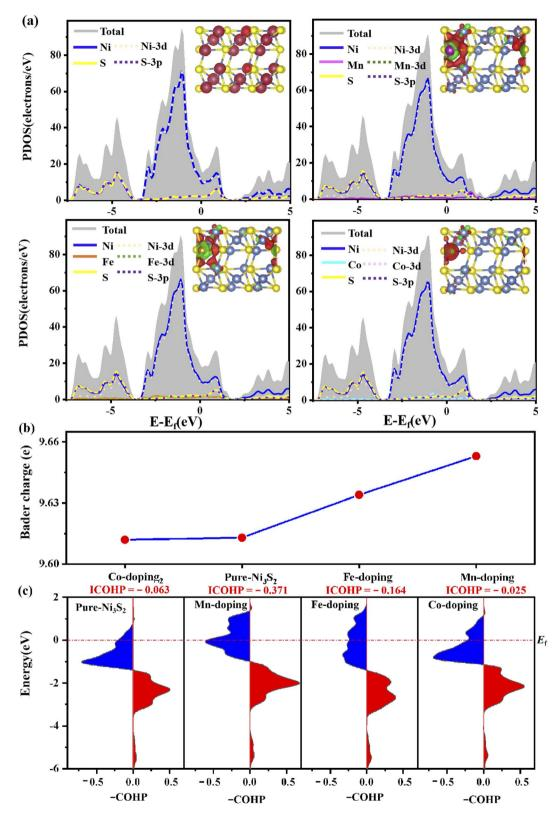
Fig. 2 (a) Partial DOS, (b) the Bader charge on the active Ni atom and (c) -COHP of TM-Ni on the pure and TM-doped Ni<sub>3</sub>S<sub>2</sub> (101) facet. The insets are charge density of pure Ni<sub>3</sub>S<sub>2</sub> and charge density difference of TM-doped Ni<sub>3</sub>S<sub>2</sub>, respectively.
