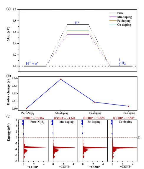
Fig. 3 (a) The  $\Delta G_{H^*}$ , (b) the Bader charge on the active-site Ni atom for hydrogen adsorption and (c) the -COHP of Ni-H in pure and TM-doped Ni<sub>3</sub>S<sub>2</sub> (101) facets.
