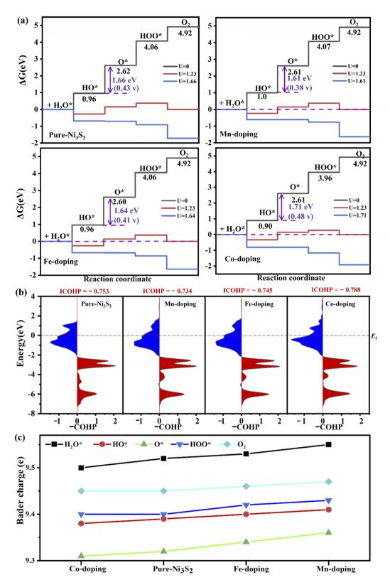
Fig. 4 (a) The free energy of four steps at different applied potentials. (b) The -COHP of Ni-O at the second step and (c) the Bader charge on the active-site Ni in pure and TM-doped Ni $_3S_2$ .
