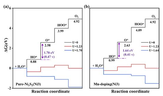
Fig. 6 The free energy of four steps for OER on (a) pure and (b) Mn-doped Ni<sub>3</sub>S<sub>2</sub> (101) facets. The Ni<sub>3</sub> atom acts as the active site.
