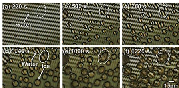
Fig. 7 Microscopic monitoring of frost formation at 5.2% RH on the MSC surface that represents the early formation of dew condensed water droplets (a) followed by continuous growth to about 15  $\mu\text{m}$  (b) and (c), partial solidification of some water droplets (d), complete solidification of all water droplets forming hoar frost around their surfaces and bridging with nearby droplets (e) and frost coalescence growth to bigger sizes on the MSC surface (f). Scale bar is 15  $\mu\text{m}$ .
