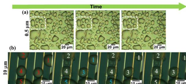
Fig. 5 Dynamic formation of ice from water droplets *via* condensation mechanism using MSC gap size of 0.5  $\mu\text{m}$  (a) and 10  $\mu\text{m}$  (b), respectively. Red numbers are for liquid water droplets, light blue numbers are for partially frozen water droplets and white numbers are for frozen water droplets.
