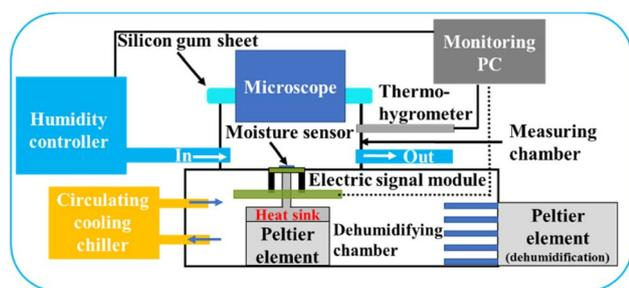
Fig. 2 A schematic illustration of the experimental setup used for frost monitoring at cooled MSC surface using microscopic water droplets in a humidity-controlled scheme.
