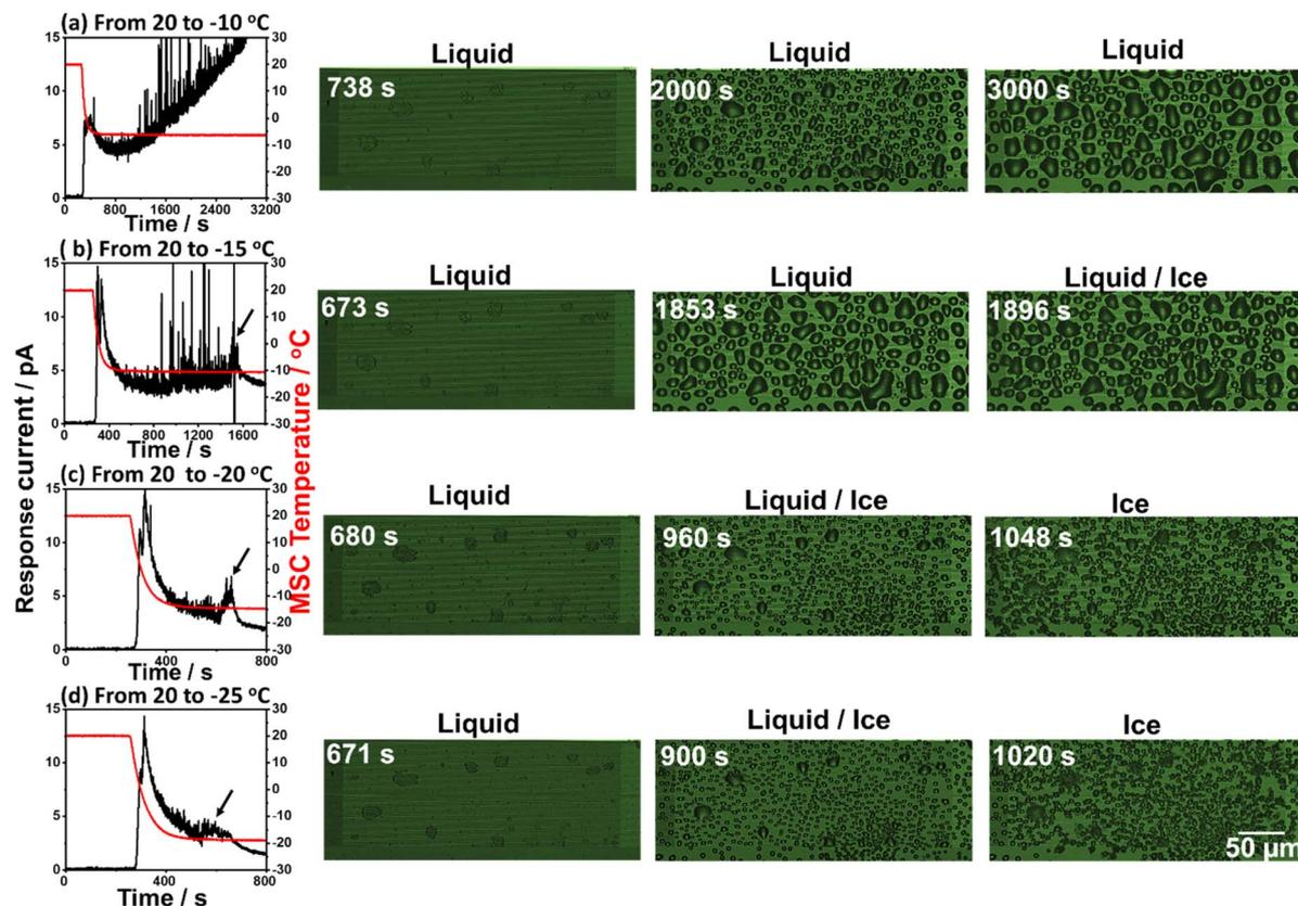
Fig. 3 Simultaneously detected galvanic response current and microscopic images during frost formation process on the surface of MSC at set temperatures of  $-10\text{ }^{\circ}\text{C}$  (a),  $-15\text{ }^{\circ}\text{C}$  (b),  $-20\text{ }^{\circ}\text{C}$  (c) and  $-25\text{ }^{\circ}\text{C}$  (d). Scale bar is  $50\text{ }\mu\text{m}$ .
