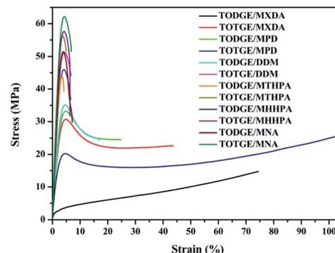
Fig. 5 Representative stress-strain curves of tung oil-based epoxy resins curing with different curing agents.
