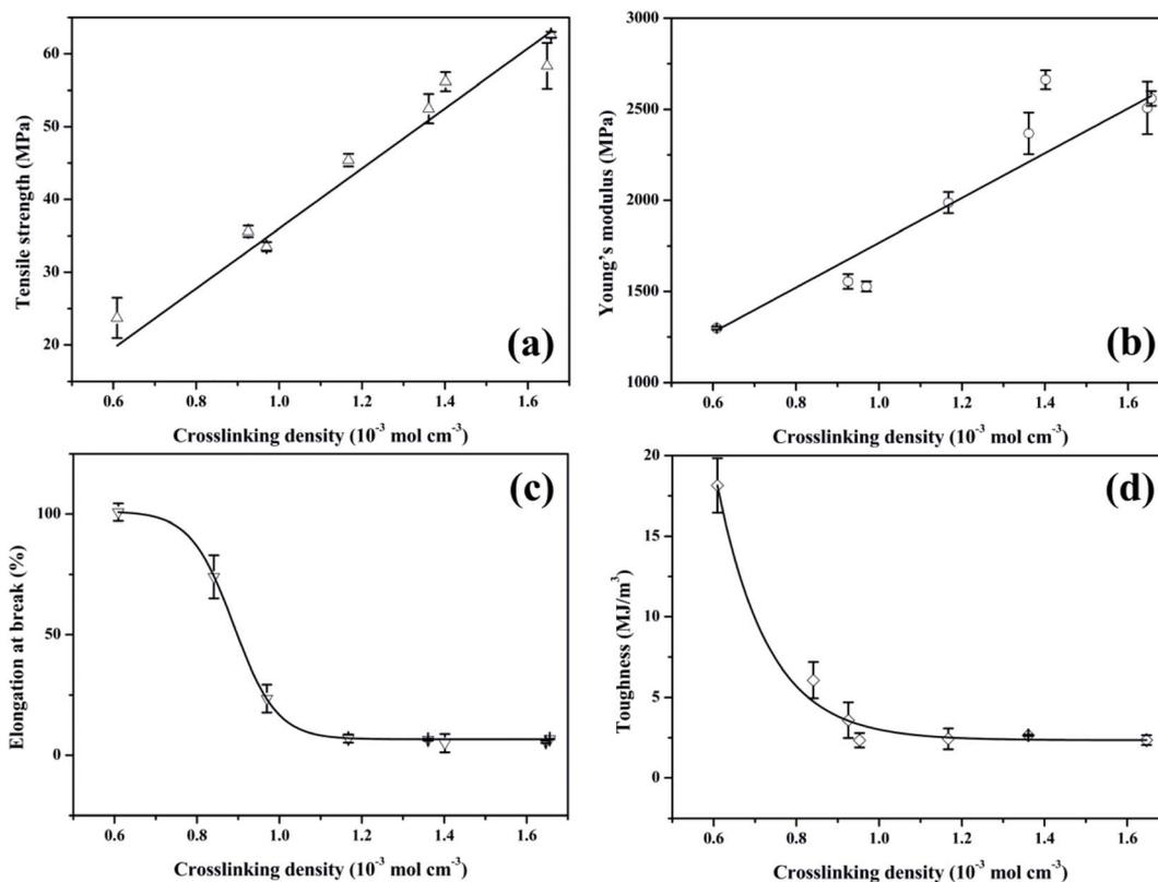
**Fig. 7** The mechanical properties of cured tung oil-based epoxy resins as a function of crosslinking density: (a) tensile strength, (b) Young's modulus, (c) elongation at break, and (d) tensile toughness.
