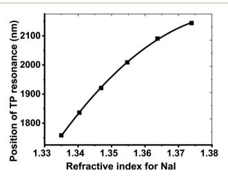
Fig. 8 The position of TP resonance as a function of refractive index for Nal solution.
