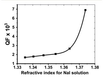
Fig. 11 The dependence of QF on the refractive index of Nal solution.
