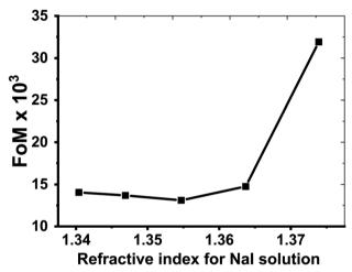
Fig. 13 The response of the figure of merit *versus* the refractive index of Nal solution.
