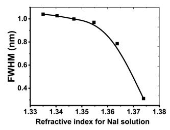
Fig. 10 The change in the values of FWHM of TP resonance with the variations in the refractive index of NaI solution.
