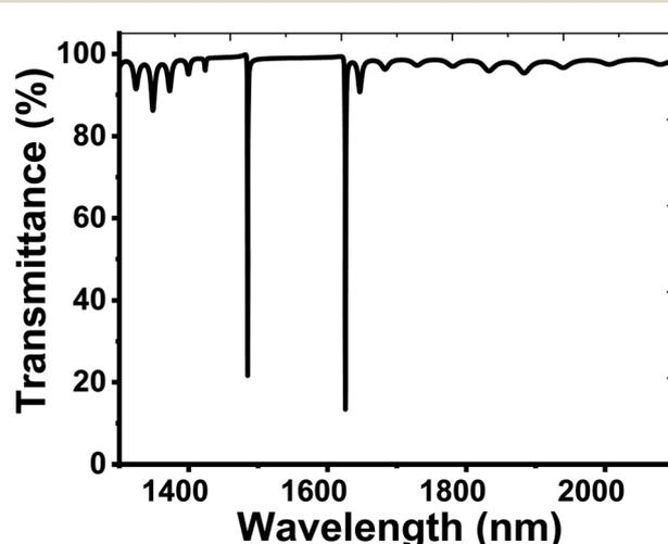
Fig. 3 The reflectance spectrum of the suggested NaI sensor that configured as, {prism/Ag/cavity/(GaN/CaF<sub>2</sub>)<sup>15</sup>/air} for normal incidence case.
