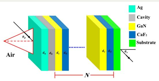
Fig. 1 The suggested design of Nal sensor that constituted as, {prism/Ag/cavity/(GaN/CaF<sub>2</sub>) <sup>15</sup>/air substrate}.
