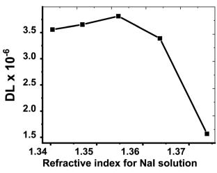
Fig. 12 The detection limit of the proposed sensor with respect to the change in the refractive index of the Nal solution.
