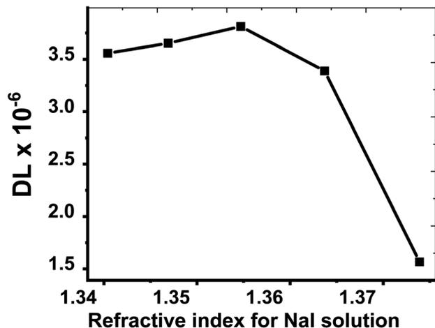
Fig. 12 The detection limit of the proposed sensor with respect to the change in the refractive index of the NaI solution.
