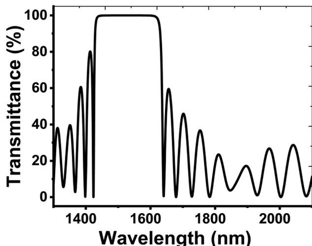
Fig. 2 The reflectivity of the suggested structure that configured as, {prism/(GaN/CaF<sub>2</sub>)<sup>15</sup>/air} in the absence of the Ag layer and for the normal incidence case.
