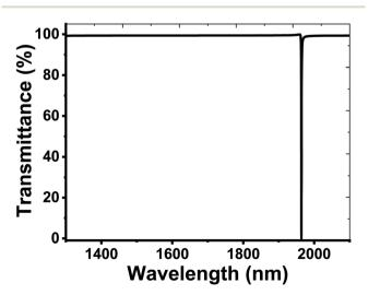
Fig. 4 The reflectivity of the proposed design in the case of the oblique incidence for TE mode of polarization at an angle of incidence  $=50^{\circ}$ .
