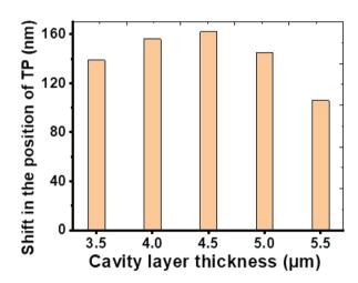
Fig. 6 The shift in the position of TP resonance mode relative to the variation in the cavity layer thickness from 3.5  $\mu$ m to 5.2  $\mu$ m.
