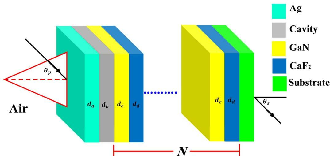
Fig. 1 The suggested design of NaI sensor that constituted as, {prism/Ag/cavity/(GaN/CaF<sub>2</sub>)<sup>15</sup>/air substrate}.
