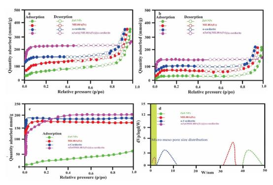
Fig. 5 N2 adsorption—desorption plot of MIL88A(Fe) MOFs, ZnO NPs, α-cordierite porous ceramic, and nZnO@MIL88A(Fe)@α-Cordierite composites before (a) and after (b) after desalination. (c) N2 simulated sorption plot of MIL88A(Fe) MOFs, ZnO NPs, α-cordierite porous ceramic, and nZnO@MIL88A(Fe)@α-cordierite composites by NLDFT model. (d) Micro-mesopore size distribution for MIL88A (Fe) MOFs, ZnO NPs, α-cordierite porous ceramic, and nZnO@MIL88A(Fe)@α-cordierite composites.
