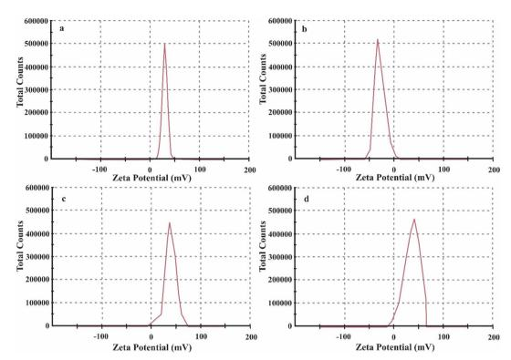
Fig. 6 Zeta potentials of ZnO NPs (a), α-cordierite porous ceramic (b), MIL88A(Fe) (c), and nZnO@MIL88A(Fe)@α-cordierite composites (d)
