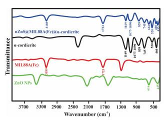
Fig. 3 FTIR patterns of ZnO NPs, MIL88A(Fe) MOFs,  $\alpha$ -cordierite porous ceramic, and nZnO@MIL88A(Fe)@ $\alpha$ -cordierite composites.
