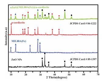
Fig. 2 XRD Patterns of ZnO NPs, MIL88A(Fe) MOFs,  $\alpha$ -cordierite porous ceramic, and nZnO@MIL88A(Fe)@ $\alpha$ -cordierite composites.
