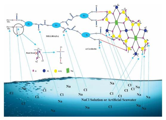
Fig. 13 The possible mechanism of adsorptive desalination.
