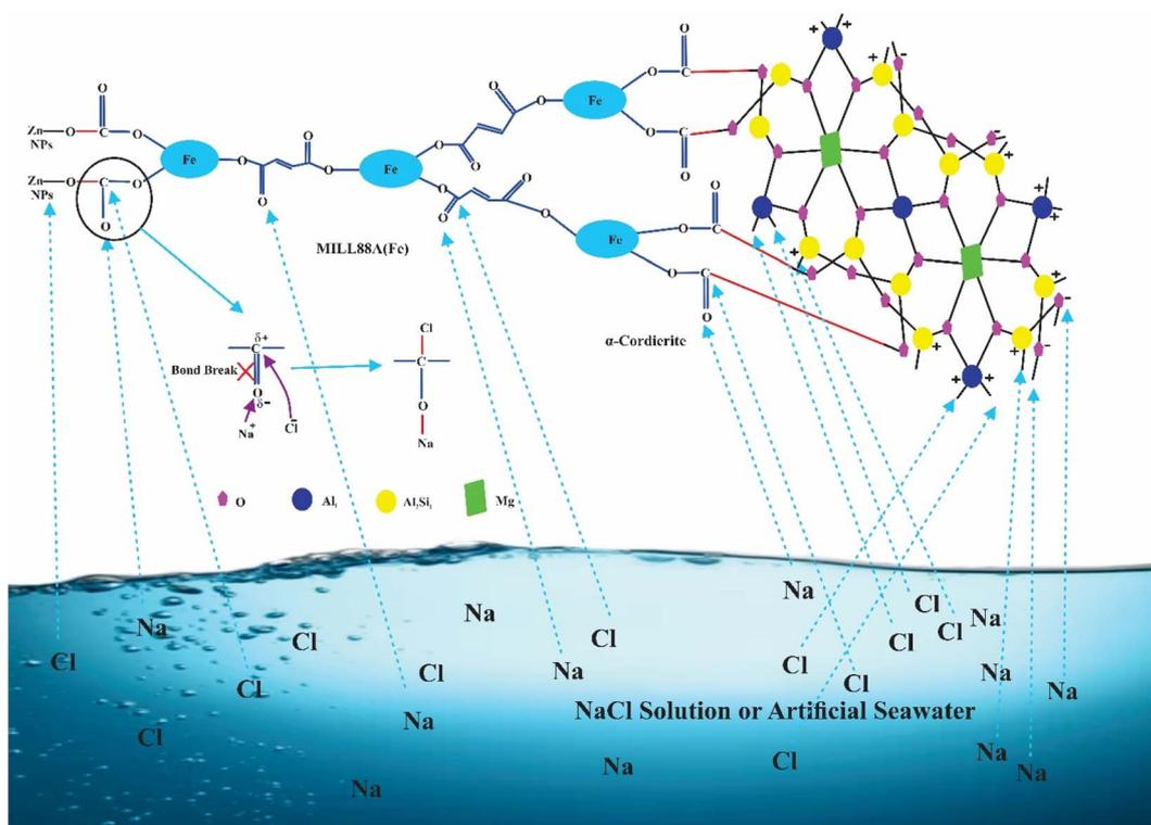
Fig. 13 The possible mechanism of adsorptive desalination.
