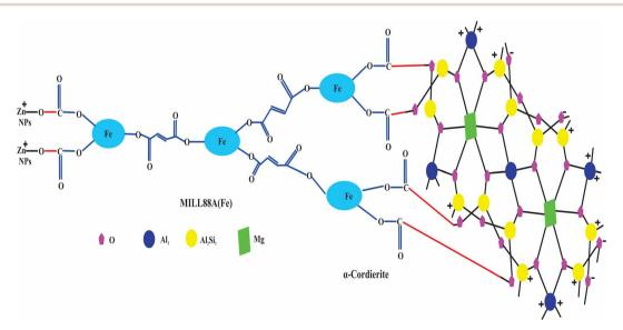
Fig. 1 Possible mechanism for synthesis of nZnO@MIL88A(Fe)@α-cordierite composites.
