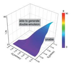
Fig. 4 Three-dimensional diagram of liquid metal double emulsion droplets formation depending on middle phase flow rate  $(Q_2)$ , outer phase flow rate  $(Q_3)$  and the inclination angle  $\theta$ . X and Y axes represent different flow variation of the phases within a certain range, while the increase of the Z axis indicates the increase of the inclination angle. The surface colored by the variable inclination angles, determines the generation of liquid metal double emulsion droplet.
