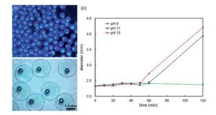
Fig. 7 Illustrations of (a-b) the morphological configuration of coreshell liquid metal hydrogel capsules after gelation with 4 wt%  $CaCl_2$  aqueous solution and (c) diameter of the spheres as a function of soaking time and pH of the surrounding solution. The scale bar is 1.0 mm in length.
