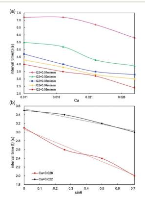
Fig. 6 Effect of (a) capillary number (Ca) of the outer phase and (b) the gravity component (denoted by  $\sin\theta$ ) on the interval time (t) of liquid metal double emulsion droplets formation. (a)  $\theta=30^\circ$ ; (b)  $Q_2=0.05$  ml min<sup>-1</sup>. The dotted lines are the linear fits of the solid lines.
